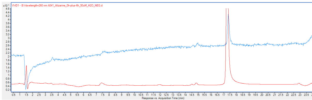
S.I. 17. Overlay of MS signal (negative ion mode) in blue and UV signal at 260 nm in red for the mixture of alizarin before and after irradiation of 6h in water at pH=12 adjusted with NH 4 OH.
