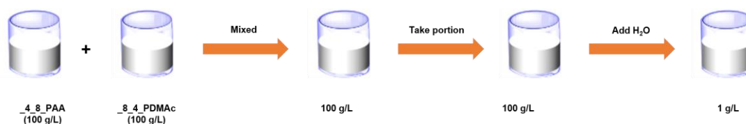
Figure 4.2.2.1. Illustration of preparation of co-assembly solution with 1 g/L.
