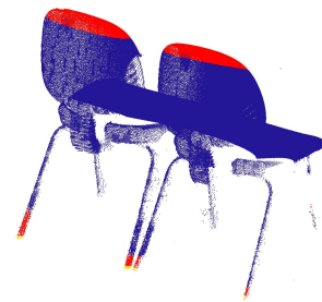
(d) Two chairs. The red color ( i.e. , “Clutter”) indicates a segmentation error in our alignment methods.
