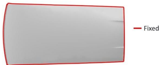
Figure 115 Fixed boundary condition applied to simulate the thermal buckling analysis of the isolated car roof.
