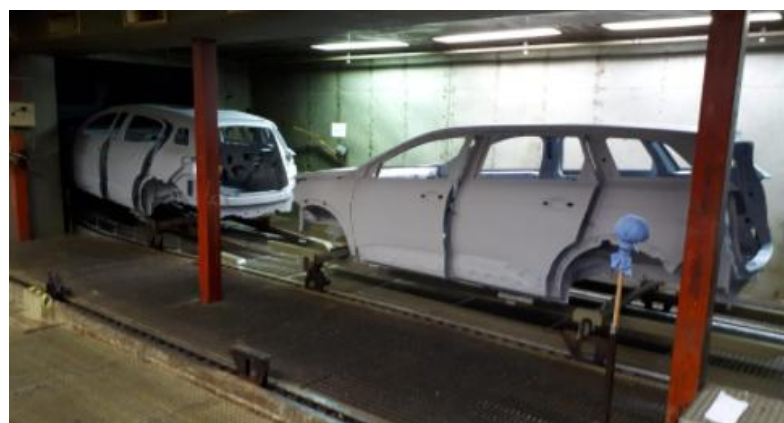
Figure 18 Body-in-white in the middle of the painting phase.
