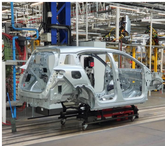
Figure 14 Body-in-white nearly complete and ready to move to the painting area.
