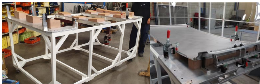
Figure 86 Tool designed to serve as a geometric reference for car roofs manufactured through stamping.
