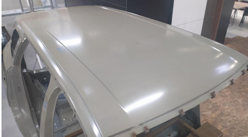
Figure 127 Modified roof after heating and cooling cycle. Material: EN AW 6056-T4 / Roof style: V3-modified.
