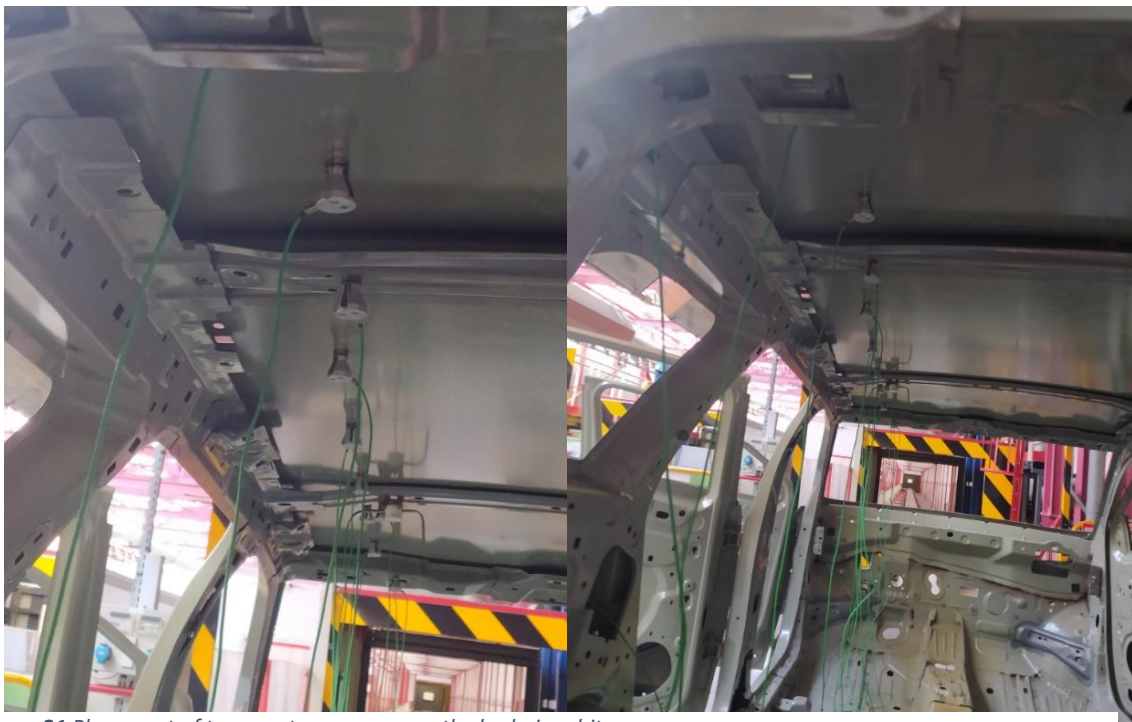
Figure 21 Placement of temperature sensors on the body-in-white
