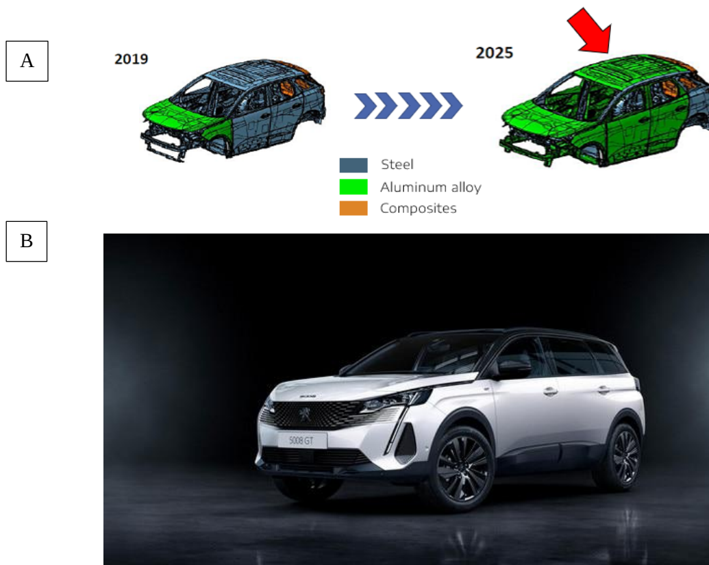
Figure 10 A) Red arrow indicating the thesis study structure and highlighting the use of aluminum alloy instead of steel; B) Picture of vehicle of study in AM2 Project (Peugeot 5008) [23].
