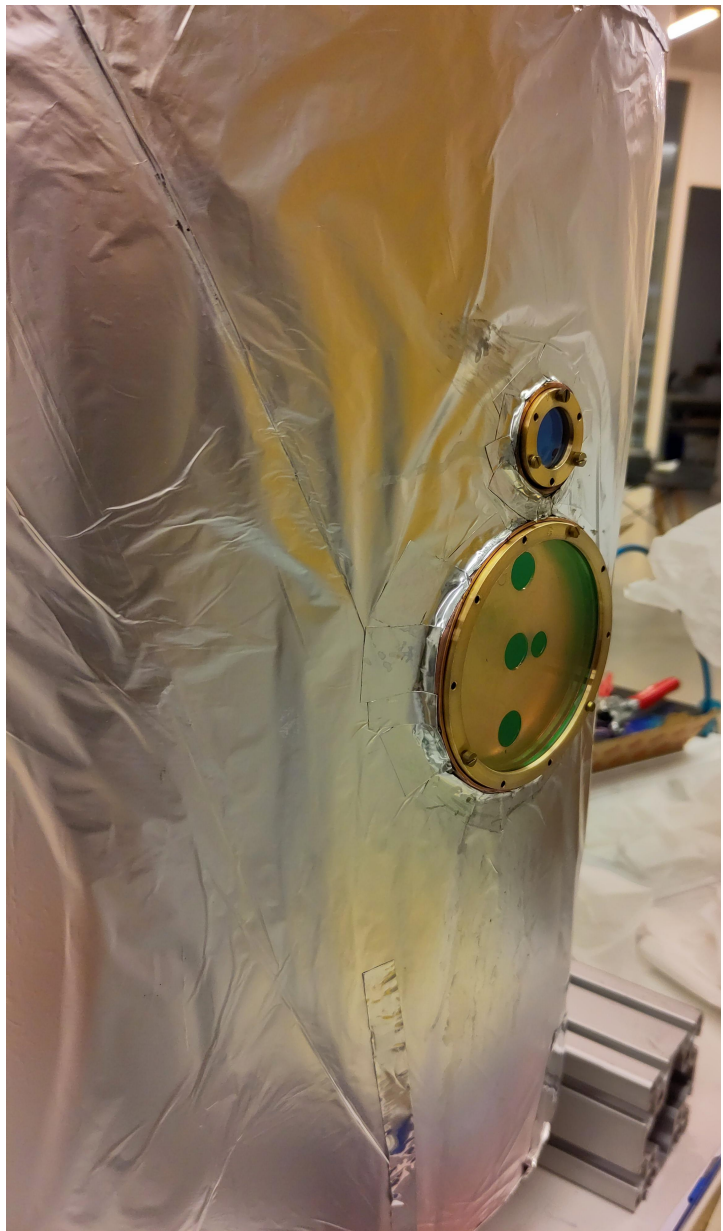
Figure 3.8. – Thermal shield windows on the helium shield. Behind the window, a copper plate with holes can be seen, used to screen the external thermal field.
