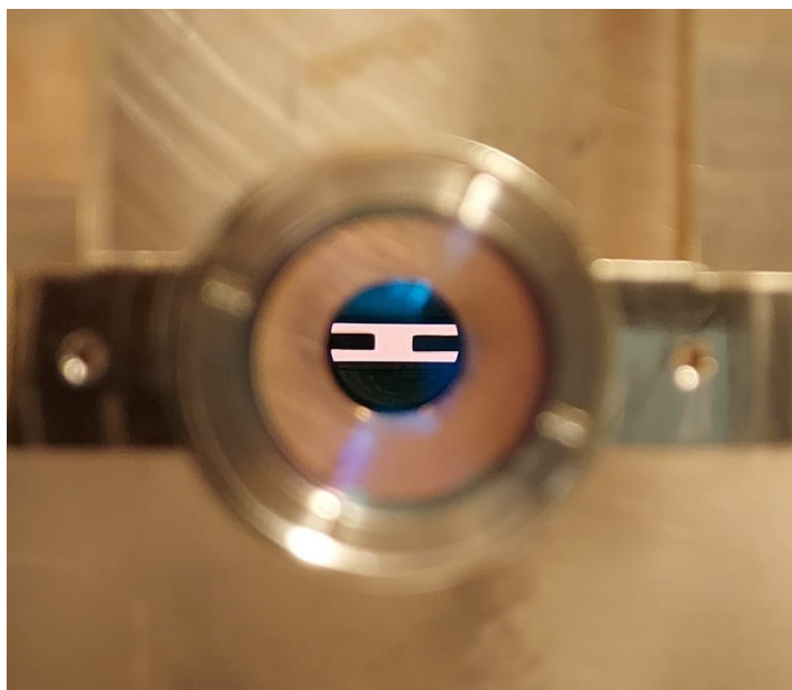
Figure 5.29. – View of the inhibition plates through the dipole trap lenses in the x direction, with the shades of the RF electrodes visible on both sides of the inhibition region.
