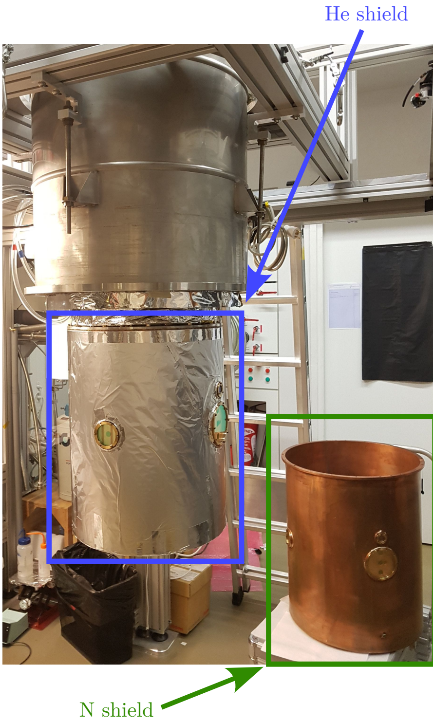
Figure 3.6. – Helium and nitrogen shields. Helium shield (blue) is wrapped with cryogenic thermal insulation and is mounted on the helium reservoir. On this picture, the nitrogen shield (green) is not yet covered with insulation and not mounted on the reservoir.
