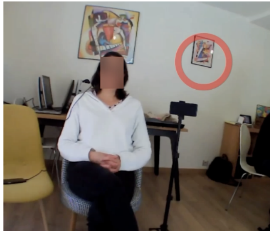
Figure 1.4. – Eye-tracking glasses were calibrated before each use by asking participants to fixate on an object in the room. The gaze marker (indicated by the red circle) was then adjusted to match the target object in real time via streaming from the camera and the gaze signal.
