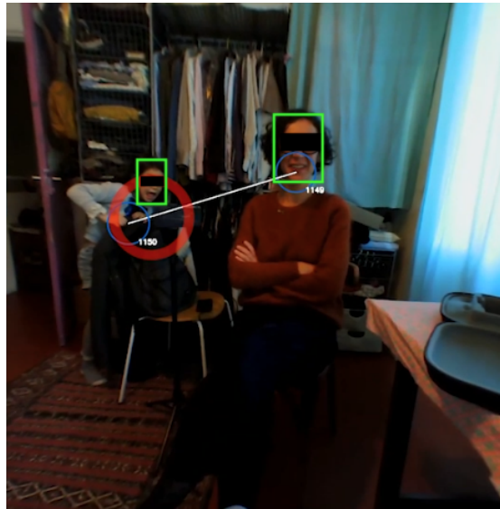
Figure 3.1. – Illustration of the RetinaFace detection and interlocutor selection process in a single egocentric frame from the Pupil Invisible glasses. The algorithm detects two faces (green bounding boxes), but only the larger one (on the right) is selected as the interlocutor based on our heuristic. The red circle indicates the most recent fixation event, and the blue circles represent previous fixations with IDs: 1149 and 1150, respectively. (Note: Faces are redacted for privacy.)
