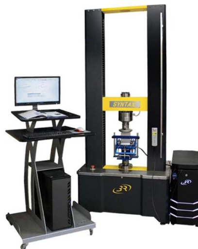
Figure 41 : Machine universelle SYNTAX 3R
