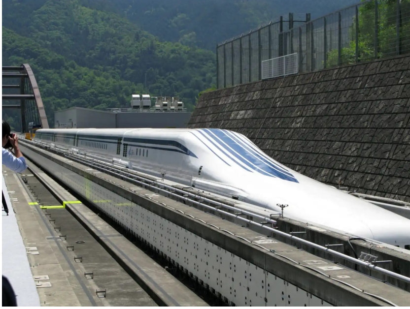
Figure 1.2: A maglev train runs along a test track in Yamanashi Prefecture, west of Tokyo, picture from Takashi Kurokawa.
