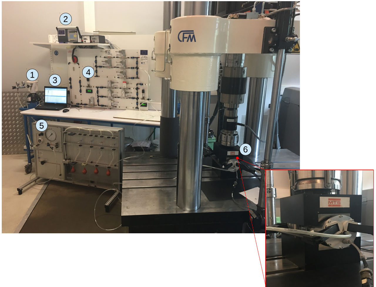
Figure 4.15: Experimental set-up of the coupling between the gas permeability and crack opening. Bottle of nitrogen with pressure regulator (1) datalogger and power (2) mass flow measur system (3) pressure gauge (4) pressure control (5) concrete specimen under applied loading and gas pressure (6).
