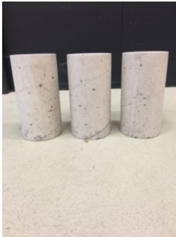
Figure 4.1: Three cylinder specimens of 110 mm of diameter and 220 mm of height with different aggregate sizes.
