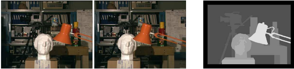
Fig. 2.10: Sample disparity map on a reference case
