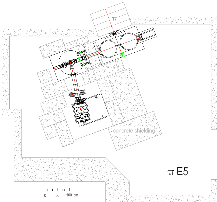
Figure 3.2 – Setup of the experiment during the 2002 measurement. The pion beam (at the top of the picture) is decelerated into the cryogenic gas target inside the cyclotron trap. X-rays from pionic atoms are reflected onto the CCD detector array by the Bragg crystal.
