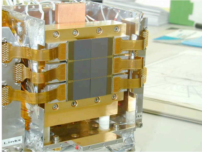
Figure 3.13 – Photo of the CCD detector array. The read-out connections are visible at the external side of each chip.
