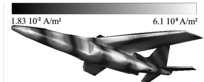
Figure B.7: Illumination of a plane by a 100MHz plane wave - Magnitude of the current density.
