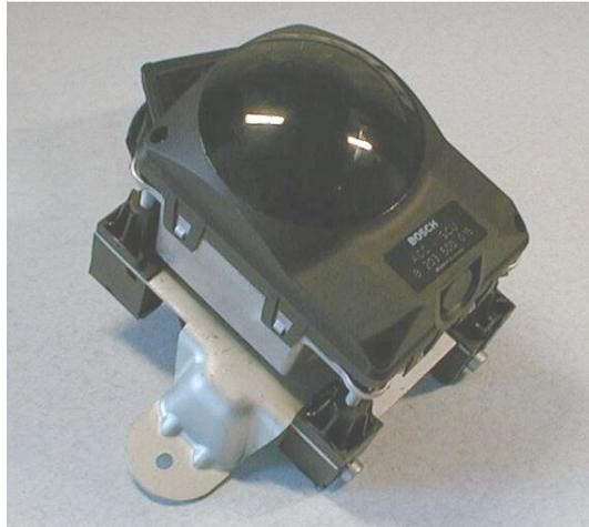
FIG. 5.4 – Radar Bosch
