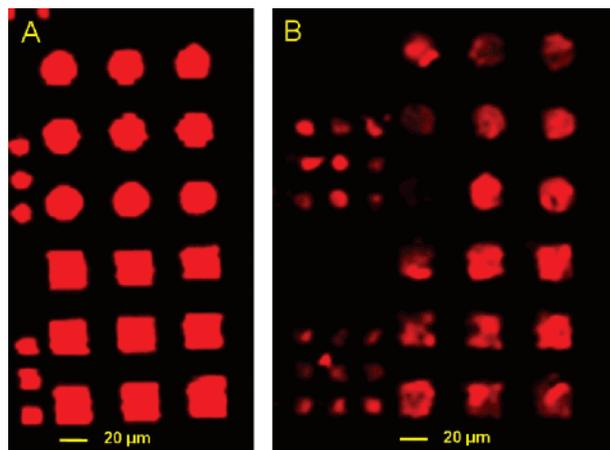
**Figure 7.** Fluorescence images of DNA spots printed by  $\mu$ CP on a glass slide. The image on the left (A) corresponds to a print achieved with an uncleaned PDMS stamp containing micrometric features compatible with fluorescence scanner characterization. The image on the right (B) corresponds to a print achieved in exactly the same conditions with a Soxhlet-cleaned PDMS stamp.
