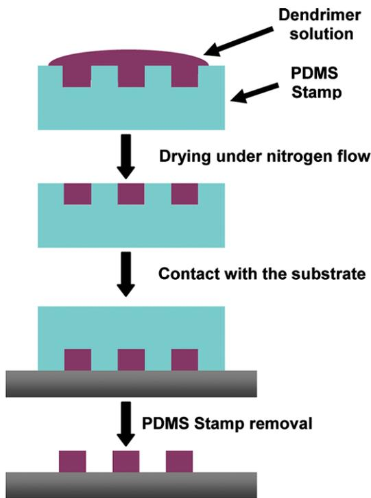
Fig. 1. Schematic procedure of microtransfer molding process.
