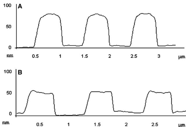
Fig. 3. AFM section of 500 nm width lines of dendrimers  $\mu\text{TM}$  on a silanised silicon wafer: (A) high concentrated solution: 60  $\mu\text{M}$  and (B) four times lower concentration: 15  $\mu\text{M}$ .
