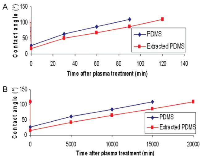
**Figure 6.** Time evolution of the water–PDMS contact angle after oxygen plasma treatment for two storing conditions: in air (A) and in water (B). Uncleaned PDMS stamps made of Sylgard material are compared to similar stamps cleaned using the Soxhlet device.
