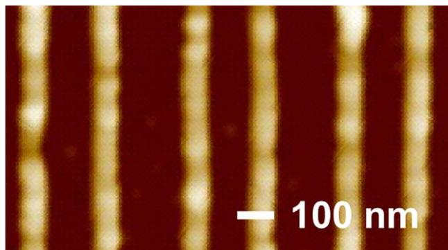
Fig. 4. Edge printing at a concentration of 6  $\mu\text{M}$ . The stamp used in this experiment is the same as for Fig. 3. Only the edges of the 500 nm lines of the stamp are transferred resulting in 100 nm wide lines and a thickness of 30 nm.
