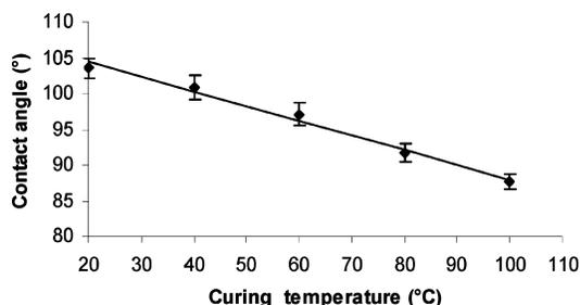
**Figure 3.** Dependence of the steady water–substrate contact angle (glass substrate) after printing with a flat PDMS stamp during 1 min as a function of the curing temperature of the PDMS material. The error bars correspond to different measurements combined with angle measurement accuracy, and the line is just a guide for the eyes.
