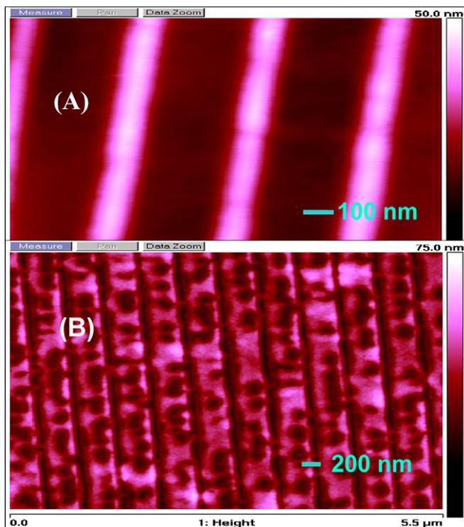
Fig. 2. (A) AFM picture of the stamp, the size of the lines are 40 nm on top of the lines. (B) AFM pictures of  $\mu\text{TM}$  dendrimer film on silicon, the lines have 40 nm widths with a pitch of 400 nm.
