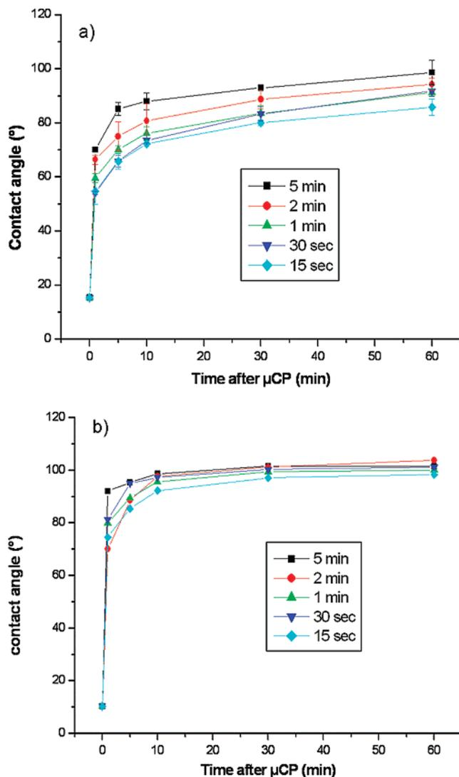
**Figure 4.** Time evolution of the water–substrate contact angle (glass substrate) after printing with flat PDMS stamps. The different experimental points correspond to various contact times ranging from 15 s to 5 min. (a) PDMS stamp made of Sylgard cured for 24 h at 60 °C and (b) PDMS stamp made of Material A cured for 2 h at 60 °C.
