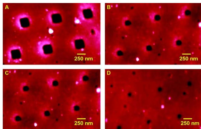
Fig. 6. AFM images of microtransfer molding of dendrimer films. All the features have a pitch of 1  $\mu\text{m}$  (A) 250 nm squares, (B) 100 nm squares, (C) 80 nm squares and (D) 50 nm squares. All the features are in negative.
