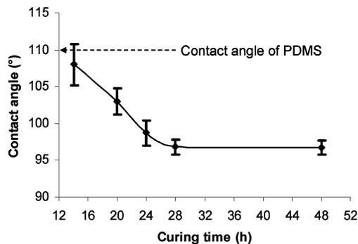
**Figure 2.** Dependence of the steady water–substrate contact angle (glass substrate) after printing with a flat PDMS stamp during 1 min as a function of the curing time of the PDMS material at 60 °C. The error bars correspond to different measurements combined with angle measurement accuracy, and the line is just a guide for the eyes. The horizontal arrow indicates the contact angle of water on bulk PDMS.
