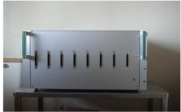
Figure 4.20: Rack blindé contenant les ampli.
