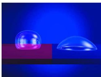
FIG. 2 – Surface hydrophobe (*gauche*)/hydrophile (*droite*)
