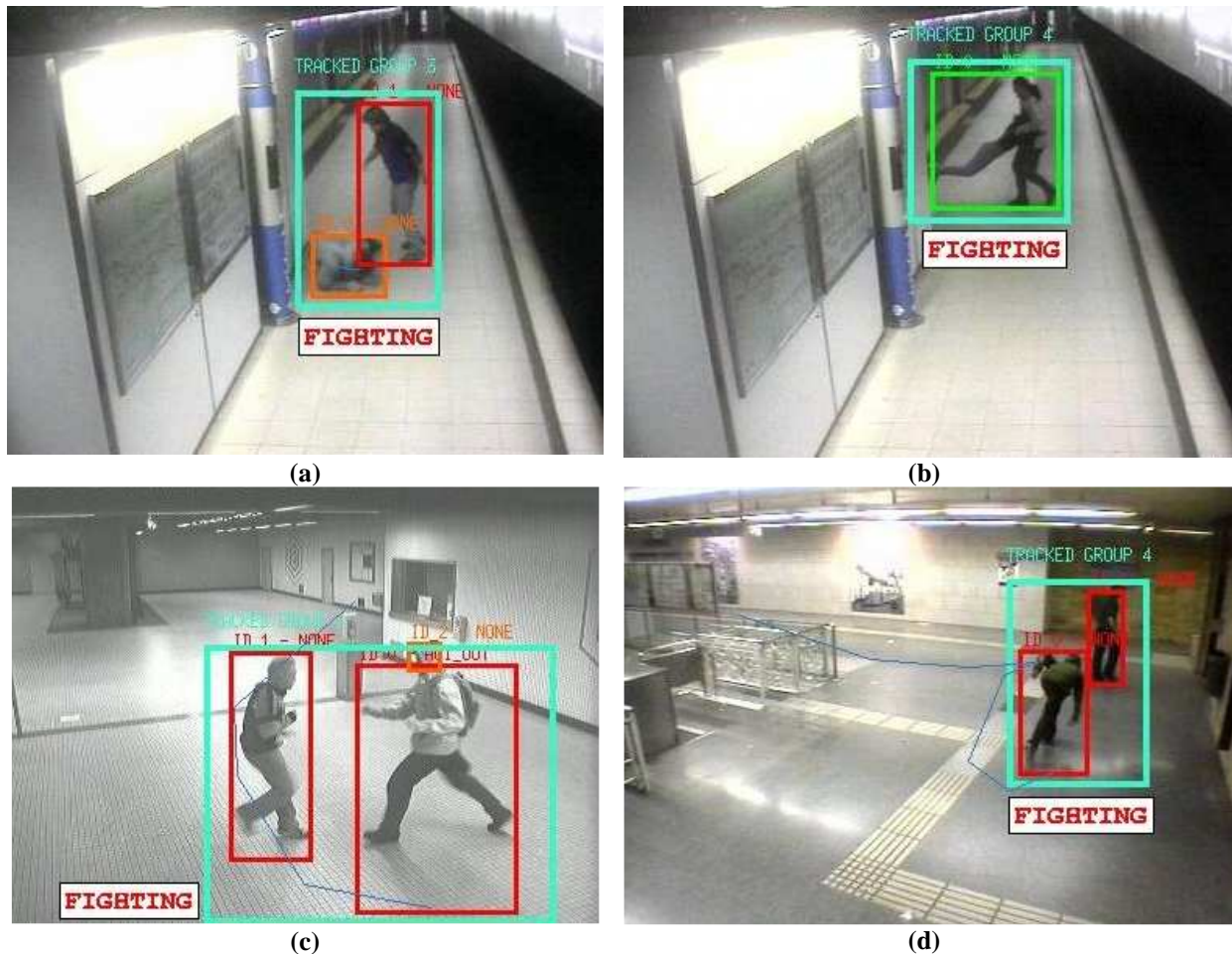
Figure 7.1: This figure illustrates four methods combined by an AND/OR tree to recognise the behaviour "Fighting". Each image illustrates a configuration where one method is more appropriate to recognise the behaviour: (a) lying person on the floor surrounded by people, (b) significant variation of the group width, (c) quick separation of people inside a group and (d) significant variation of the group trajectory.
