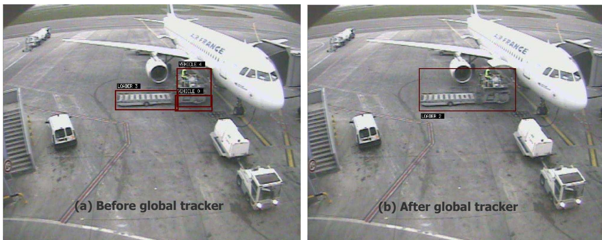
Figure 6.2: On the left, a Loader vehicle is detected as several mobile objects (over detection) while on the right, the Loader vehicle is correctly tracked as one mobile object.
