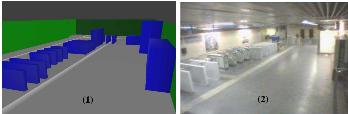
Figure 9.4: Sagrada-Familia station in Barcelona: (1) raw image taken by a camera and (2) scene context model corresponding to this image.
