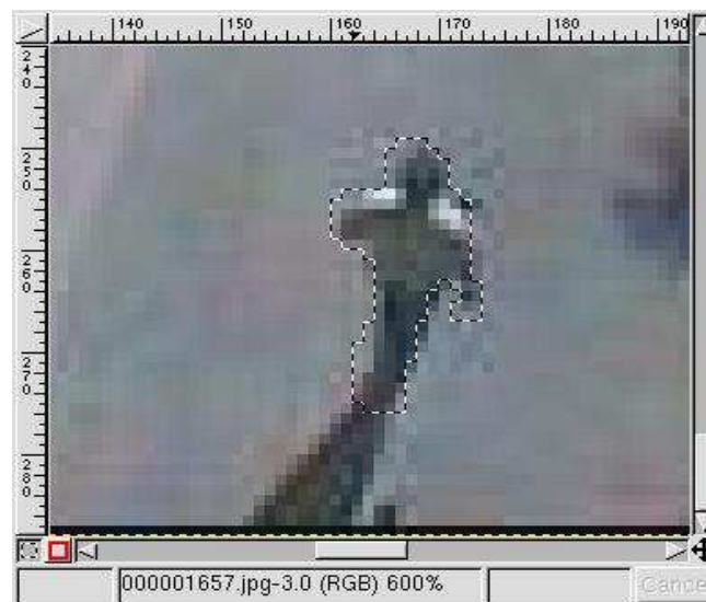
Figure 8.8 : Definition of the shape of a physical object of interest to obtain a pixel-based ground truth.
