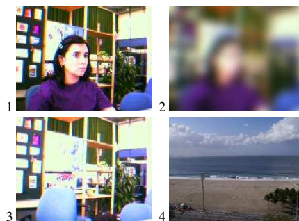
Figure 6: Nimbus control: image captured by the camera (1), filtered image (2), ambiguous pre-recorded image (3) and explicit absence indicator (4).
