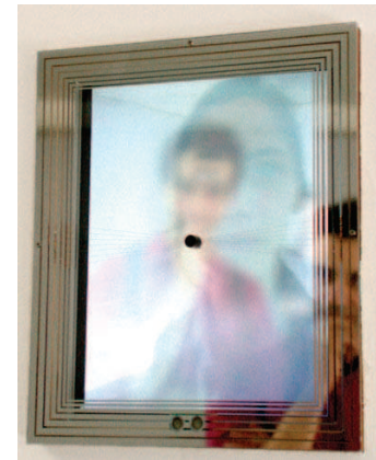
Figure 6. Close up showing the proximity (bottom) and image sensors (center).
