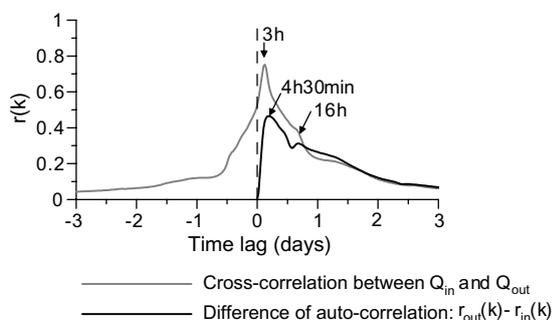
**Figure 8** Correlation analysis between the discharge in the G1 gauging station and the discharge in the G2 gauging station using all the available data (33months).  $\{k = 30\text{ min}, m = 96\text{ h}\}$ .
