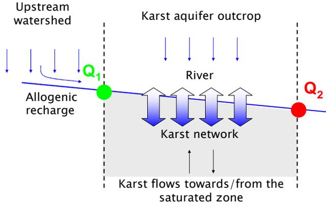
**Fig. 85: Karst/River interaction in case of allogenic stream**
