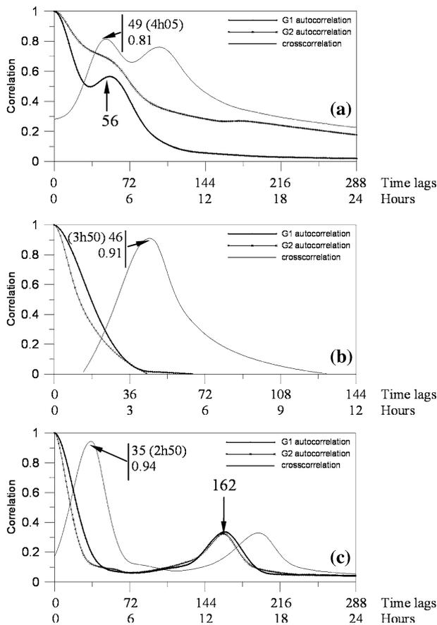
**Fig. 5** **a** Autocorrelation functions and crosscorrelation function computed with the flood 1. **b** Autocorrelation functions and crosscorrelation function computed with the flood 2. **c** Autocorrelation functions and crosscorrelation function computed with the flood 3
