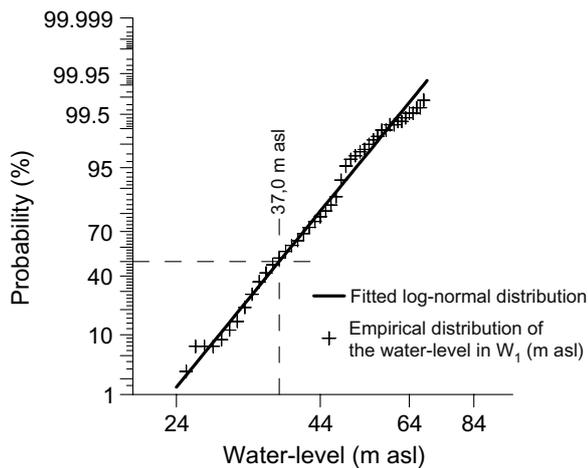
**Figure 3** Statistical distribution of the water-level measured in  $W_1$ . Probability is the cumulative percentage of the water-level measurements fitted to a log-normal distribution.
