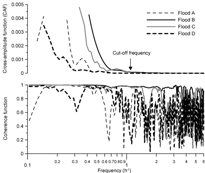
**Figure 13** Cross-amplitude functions and coherence functions computed for each flood event between the discharge in the G1 gauging station and the discharge in the G2 gauging station.  $\{k = 5 \text{ min}, m = 24 \text{ h}\}$ .
