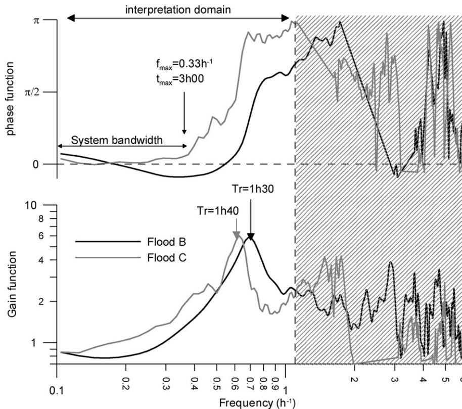
**Figure 14** Frequency response of the system computed for each flood event between the discharge in the G1 gauging station and the discharge in the G2 gauging station after phase synchronization.  $\{k = 5 \text{ min}, m = 24 \text{ h}\}$ .
