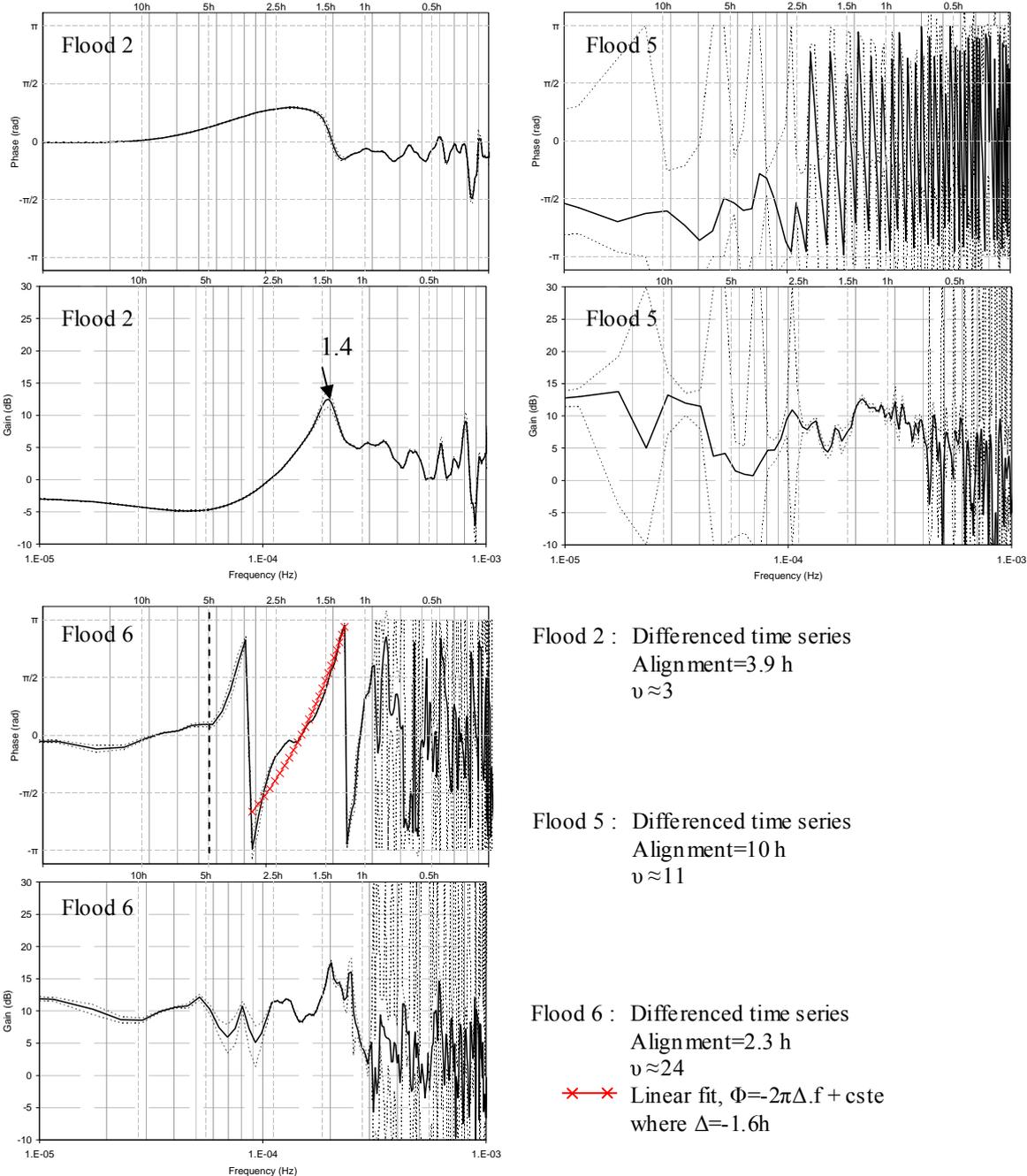
**Fig. 90:**  $Q_1/Q_2$  frequency response function using both aligned and differenced data,  $k=5\text{min}$ ,  $m=24\text{h}$ , floods 2, 5, and 6; black dashed lines represent the 95% confidence interval.
