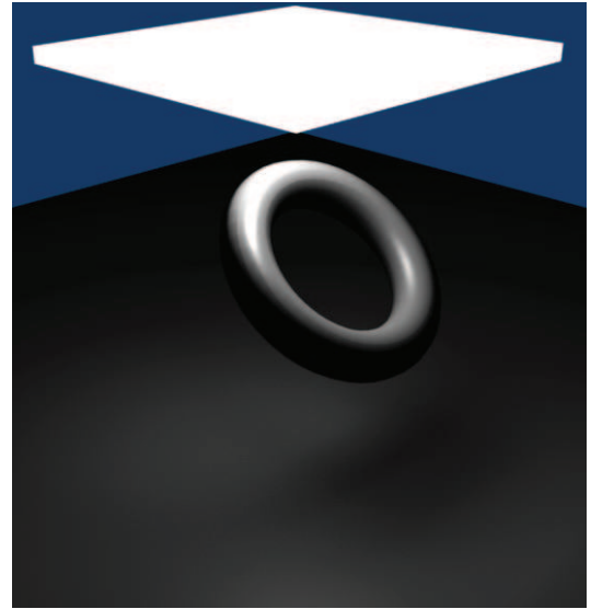
Fig. 10.2 : A very large source leads to soft shadows. All points on the floor are actually lit
