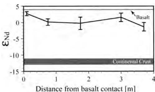
**Fig. 8.** The evolution of the Nd isotopic compositions with distance in the salt profile together with the compositions of average basalt and average continental crust. The error bars represent  $\pm 2$  sigma mean values of the individual measurements.
