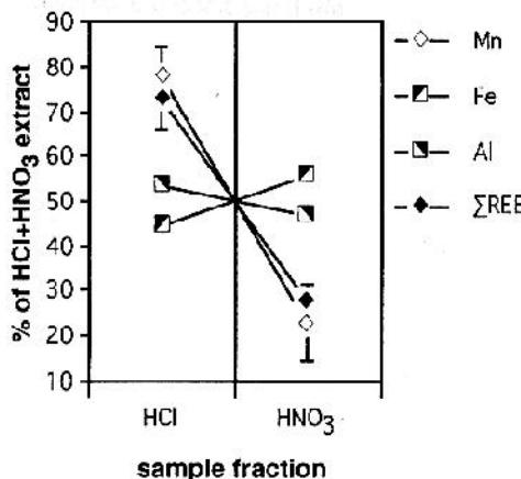
Fig. 9. Proportions of Mn, Fe, Al and REE extracted in the HCl and  $\text{HNO}_3$  step (absolute amounts of element in  $\text{HCl} + \text{element in } \text{HNO}_3 = 100\%$ ). The values given are averages of all samples with standard deviations. Only Mn shows a similar percentage change between the two extraction steps as the REE.
