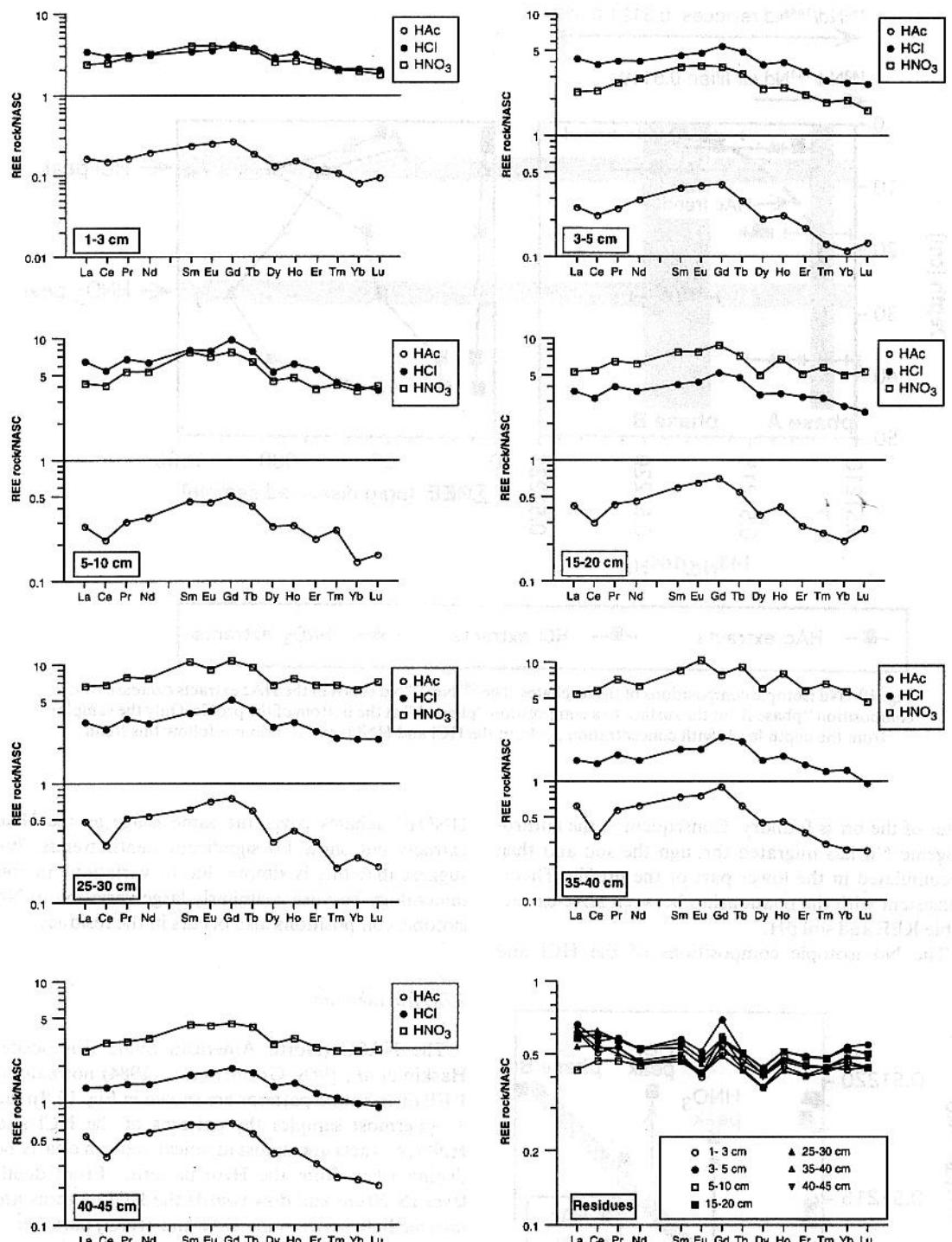
Fig. 12. NASC (North American Shale Composite) normalized REE distribution patterns of the leachates at different depth levels and the residues. Before the NASC normalization the REE concentrations of the leachates were in  $\mu\text{g/g}$  dissolved sample, and those of the residues in  $\mu\text{g/g}$  residue, in order to characterize the leached and the residual phases.
