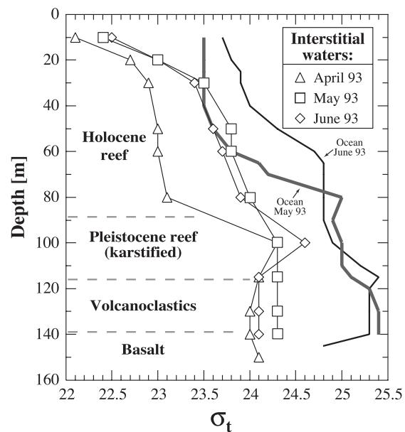
Fig. 3.  $\sigma_t$  values for the interstitial fluids of April to June 1993 in comparison with seawater values from the immediate vicinity of P ( $\sigma_t = \{\text{density} - 1\} * 1000$ ). The interstitial fluids are, in particular below 60 m, systematically lighter than seawater. The  $\sigma_t$  values have been determined with a T-S diagram and are based on the temperature and salinity data given in Tables 2 and 3.
