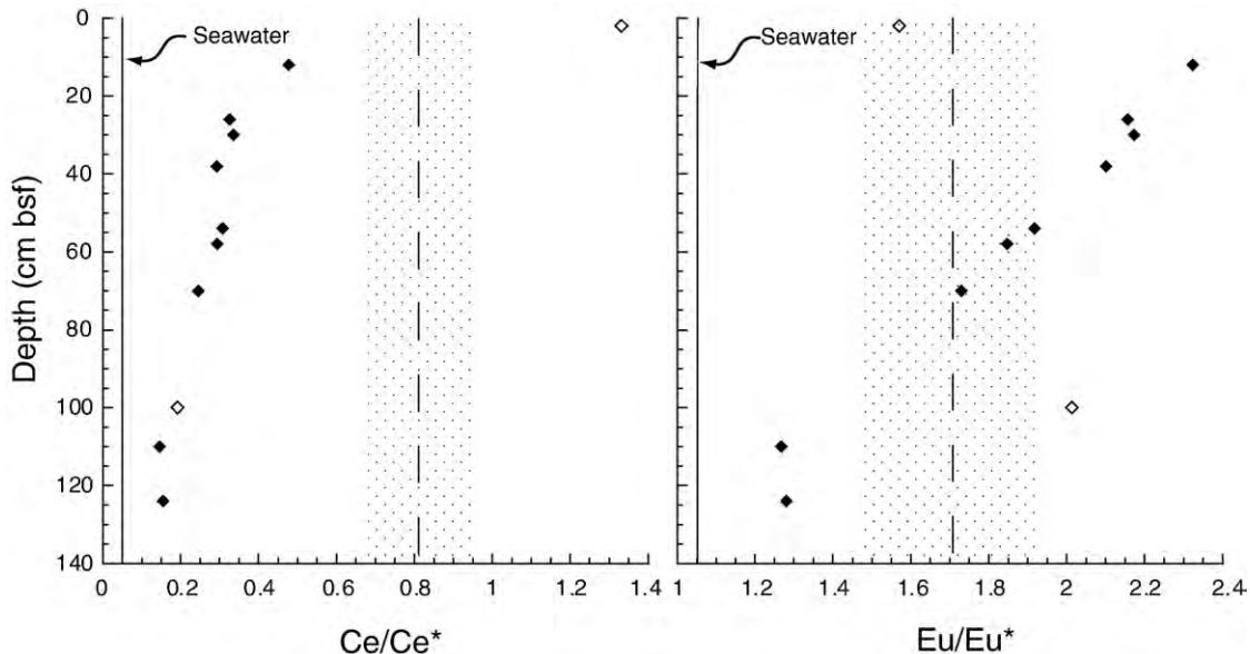
Fig. 10. Ce/Ce\* and Eu/Eu\* changes with depth for all GC50 samples. The solid lines = seawater values; dotted lines = average of the reference samples with the standard deviation. Open filled = surface nodule at 2 cm bsf and non-indurated Mn oxide layer at 100 cm bsf.
