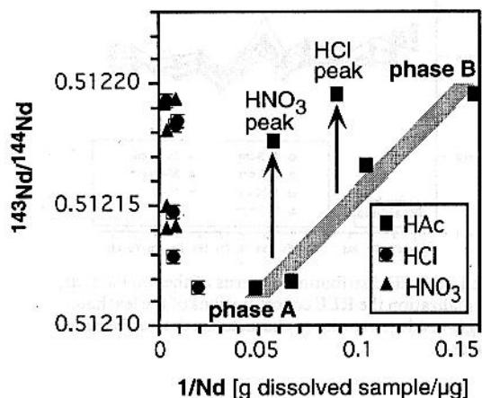
Fig. 11. Nd mixing diagram. The HAc extracts describe a mixing line between phase A and phase B. The two samples from the depth levels with concentration peaks in the HCl and  $\text{HNO}_3$  extracts are shifted towards higher Nd isotopic compositions. We suggest that phase A is dominated by anthropogenic and phase B by natural Nd.
