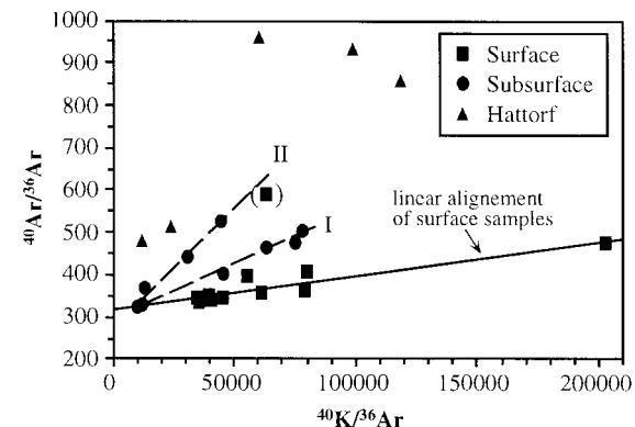
Fig. 10. K–Ar isochron diagram with all surface and subsurface samples including the Hattorf dyke. Note the lower <sup>40</sup>Ar/<sup>36</sup>Ar values for the surface samples and their linear alignment. See text for the alignments labelled I and II.
