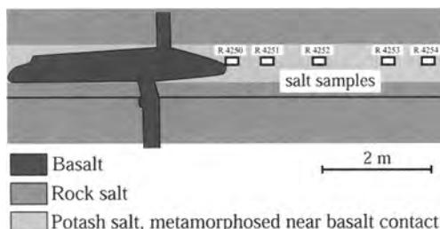
**Fig. 2.** The salt profile studied here is situated next to a basalt dyke, which is locally enlarged to an apophysis. The sampling points in the salt are indicated by the small rectangles numbered R 4250 to R 4254.
