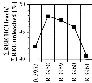
Fig. 6. Rare earths removed in the Hattorf dyke profile by leaching with 1.5 M HCl relative to the REE content in the  $\text{H}_2\text{O}$ -washed whole rock samples.
