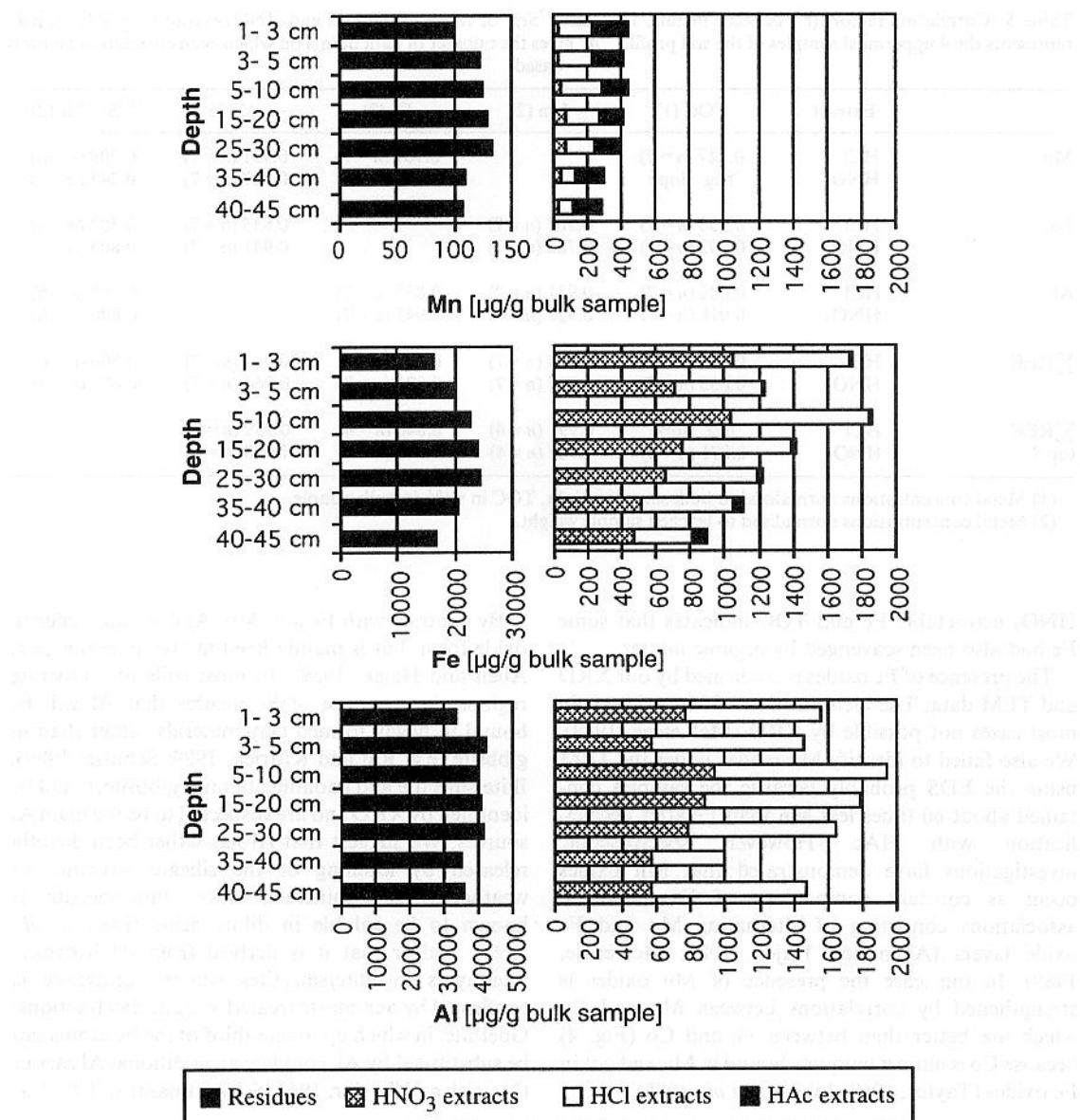
Fig. 3. Mn, Fe and Al concentrations in the extracts and the residues. All concentrations are normalized to initial bulk sample weight in order to illustrate the total amounts extracted in the different steps and to compare them with the concentrations remaining in the residues.
