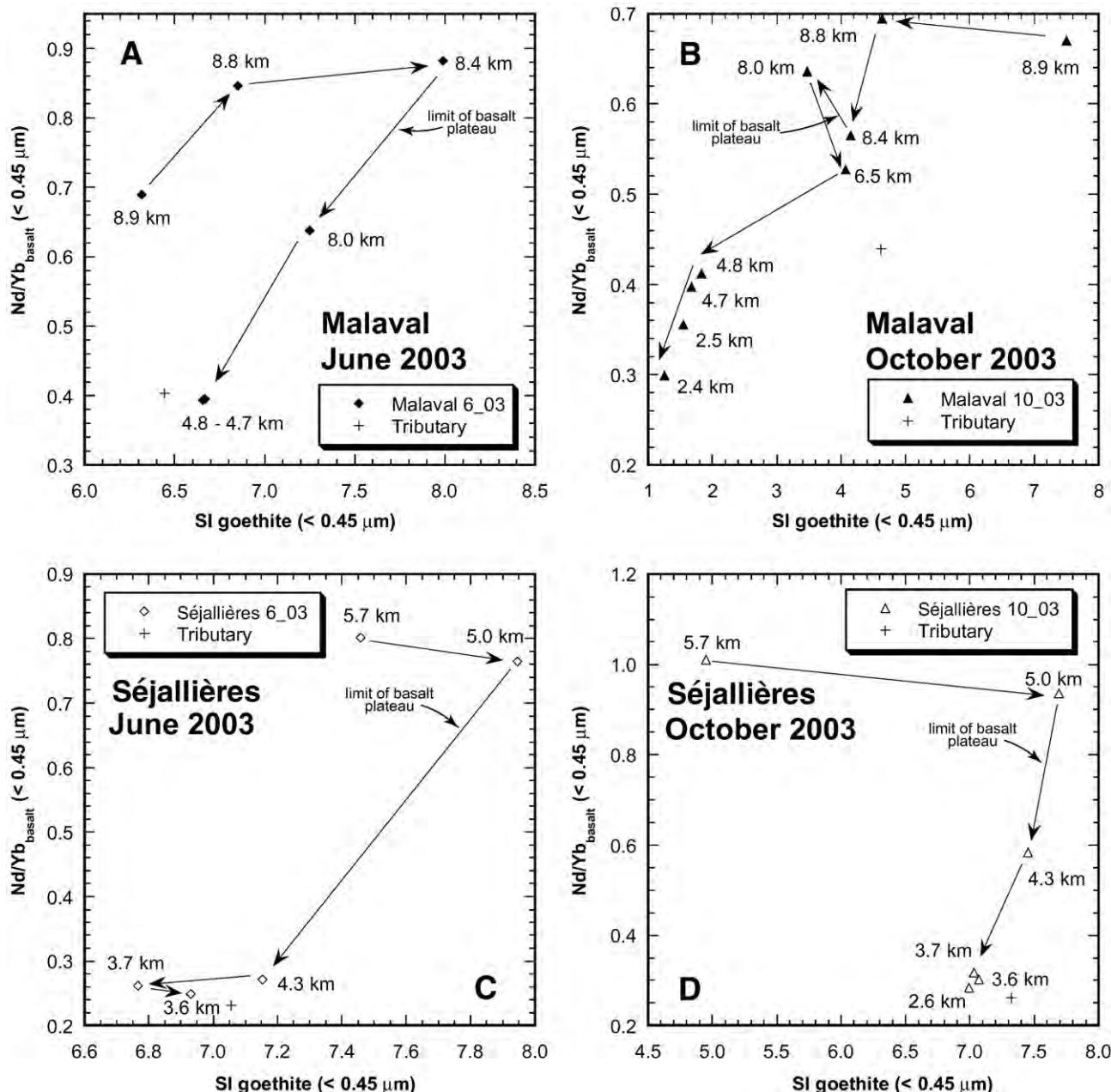
**Fig. 7.** Plots of Nd/Yb ratios vs saturation index (SI) of goethite for the <0.45  $\mu\text{m}$ . Both values decrease systematically from upstream to downstream suggesting that goethite particles are removed from the <0.45  $\mu\text{m}$  fraction scavenging preferentially the light REE such as Nd whereas Yb and the other heavy REE remain in solution.
