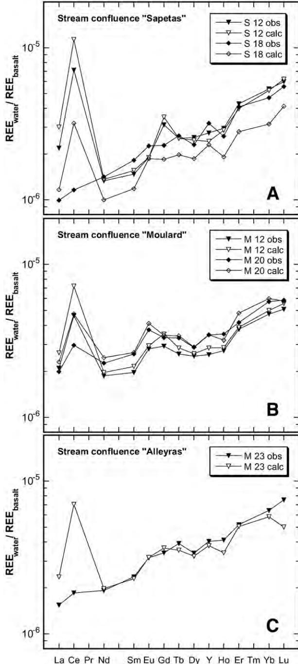
**Fig. 8.** Comparison between observed and calculated REE patterns from the stream confluences “Sapetas”, “Moulard”, and “Alleyras”. Note that Ce anomalies are systematically more positive for the calculated patterns indicating that Ce is removed from solution during water mixing at stream confluences.
