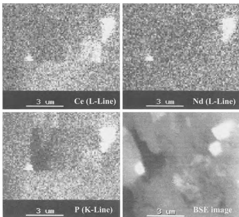
**Fig. 6.** Element maps of Ce, Nd, and P demonstrating the high REE content of the secondary apatite. The elevated REE concentrations lead to the high contrast of the apatite in the backscattered electron (BSE) image.
