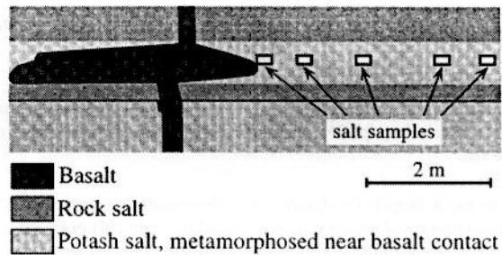
**Figure 1.** The salt profile studied here is situated in a underground mine next to a basalt dyke which is locally enlarged to an apophysis.
