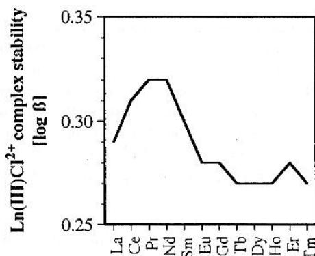
**Figure 4.** Plot of the complex stability constants of  $\text{Ln}(\text{III})\text{Cl}^{2+}$  complexes. They give, except for Yb and Lu, an inverse mirror image of the REE distribution patterns of the samples R 4253 and R 4254 shown in figure 2. The stability constants are infinite dilution values from Millero (1992) and given in table III. The values for Yb and Lu are below 0.25 and not shown to limit the scale of the figure (Yb = 0.16; Lu = -0.03).
