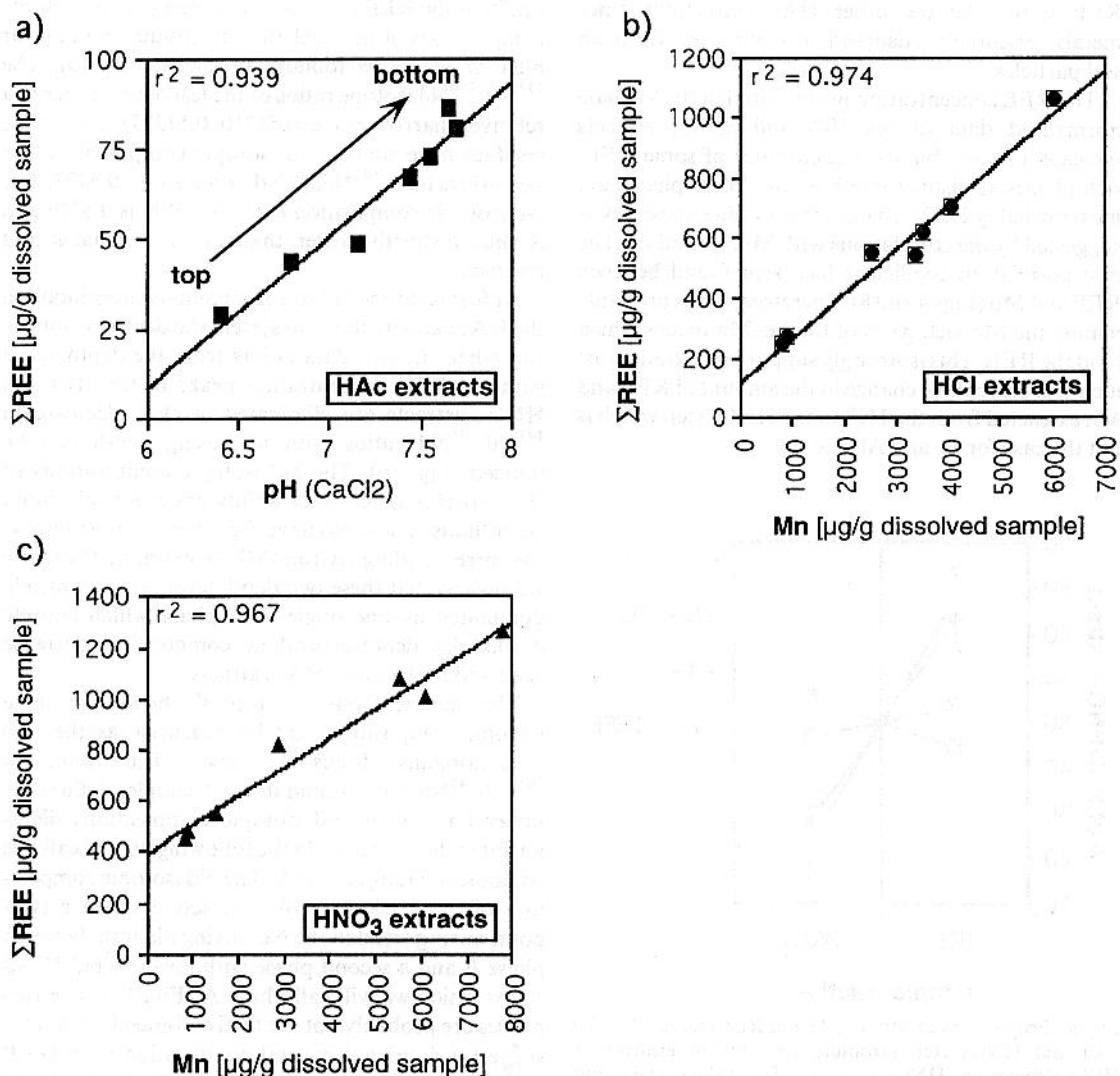
Fig. 8. The HAc extractable REE are correlated with soil pH whereas the REE of the HCl and HNO<sub>3</sub> extracts are correlated with Mn.
