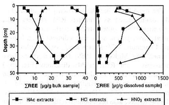
Fig. 7. Depth distribution of REE concentrations. The difference between the two diagrams is the different normalizations. The diagram on the left describes the total amount of REE extracted in each step whereas the diagram on the right shows the concentrations in the extracted phases.
