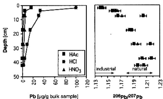
Fig. 5. The  $^{206}\text{Pb}/^{207}\text{Pb}$  isotope ratios demonstrate the retention of anthropogenic Pb in the uppermost 30 cm. Pb concentrations are bulk sample normalized in order to illustrate the absolute amounts of Pb extracted. The limits of the industrial and natural  $^{206}\text{Pb}/^{207}\text{Pb}$  ranges are discussed in the text.
