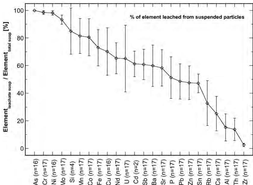
**Fig. 2.** Average percentage with standard deviation of trace elements removed from the particle fraction by leaching with HCl 1 M. The average values are based on percentages calculated for each individual sample by the formula % leached = 100 \* {conc leachate/(conc leachate+conc residue)}.
