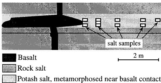
Fig. 2. The salt profiles studied here are situated in an underground mine next to a basalt dyke which is locally enlarged to an apophysis. The sample numbers and the exact distances from the basalt contact are given in Table 1. No vertical exaggeration.
