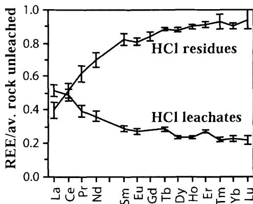
**Fig. 4.** Average REE concentrations with standard deviations of the 5 HCl leachates and residues normalized to the average concentrations of the H<sub>2</sub>O-washed whole rock.
