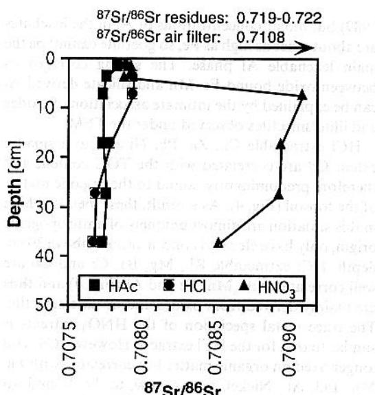
Fig. 6. Depth distribution of the Sr isotopic compositions of the leachates. Analytical errors are smaller than symbol widths. The indicated depth scale is arbitrary. The sharp increase in the Sr isotopic composition of the HCl and  $\text{HNO}_3$  extracts with its lower carbonate content could reflect another Sr source.
