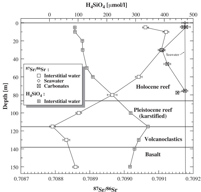
Fig. 5. Depth profiles of dissolved silica and  $^{87}\text{Sr}/^{86}\text{Sr}$  of interstitial fluids, and  $^{87}\text{Sr}/^{86}\text{Sr}$  of seawater and reef carbonates. The interstitial fluids have been sampled on 15th June 1993. Note the opposite depth evolutions of silica and  $^{87}\text{Sr}/^{86}\text{Sr}$  for the interstitial fluids. The  $^{87}\text{Sr}/^{86}\text{Sr}$  seawater values are based on the data points from 0 and 500 m. See Table 4 for raw data.
