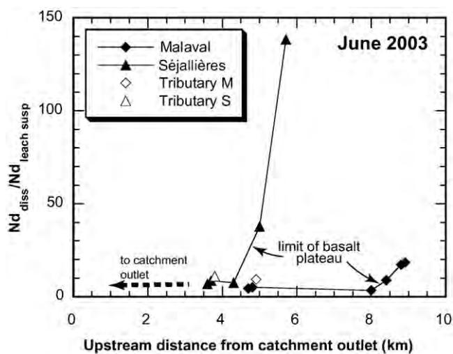
**Fig. 6.** Nd concentration ratios between the  $<0.45\text{ }\mu\text{m}$  fraction over leachate particulate fraction for the sample series from June 2003. The decreasing ratios from upstream to downstream suggest a REE transfer from the  $<0.45\text{ }\mu\text{m}$  fraction to the adsorbed particle fraction.
