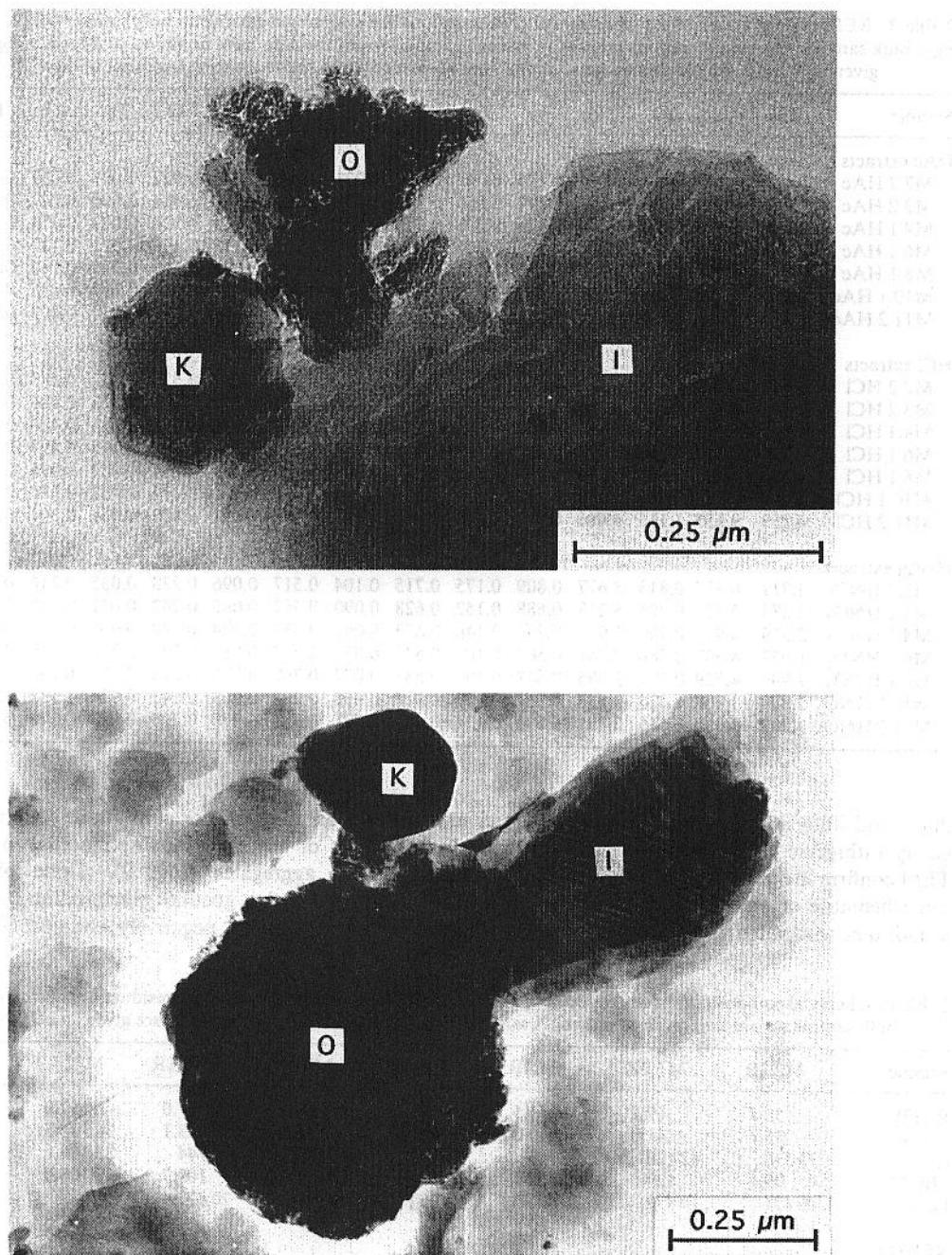
Fig. 2. TEM photographs of clay minerals (I = illite or illite/smectite, K = kaolinite) and associated Fe-Mn oxides (O) in decalcified bulk samples. Illites and illite/smectites are indistinguishable under the TEM. Note the idiomorphous hexagonal shape of the kaolinites which indicates an authigenic origin whereas the illites or illite/smectites with their rugged morphology are detrital (top: sample M4.1; bottom: sample M6.1).
