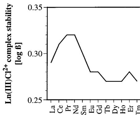
Fig. 9. Plot of the complex stability constants of  $\text{Ln}(\text{III})\text{Cl}^{2+}$  lanthanide complexes. The constants are infinite dilution values from Millero (1992). The values for Yb and Lu are below 0.25 and not shown to limit the scale of the figure ( $\text{Yb}=0.16$ ;  $\text{Lu}=-0.03$ ).
