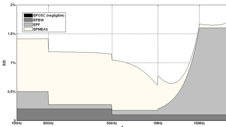
Fig. 4.12 - Agilent 4294A decomposed relative error function E(f)
