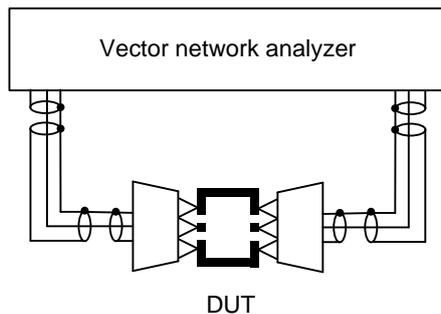
Fig. 4.14 – Vector network analyzer probing system
