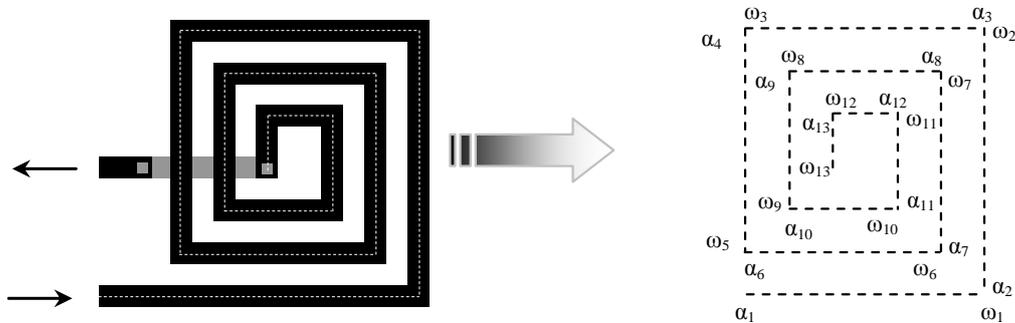
Fig. 5.6 - Equivalent topology of planar inductance
