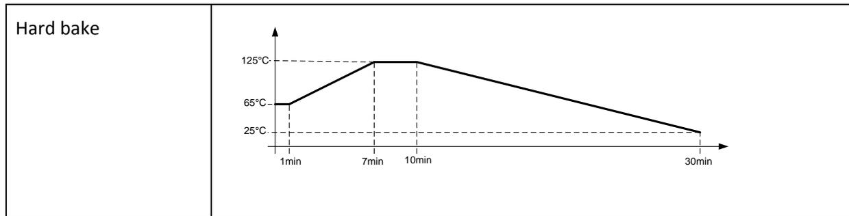
Fig. 4.2 - 5µm thick SU8 layer detailed process
