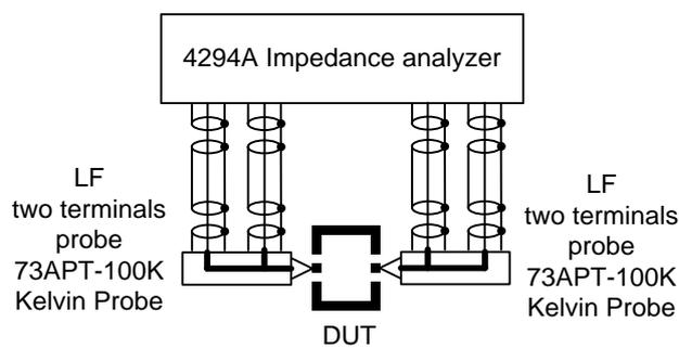
**Fig. 4.8 - Four points measurement probing system**
