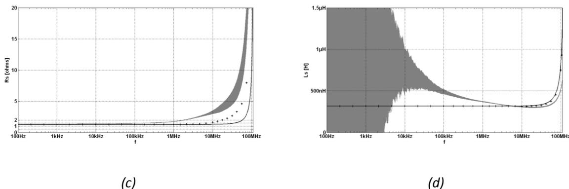
**Fig. 4.19 - Measurement of T8 inductor prototype with uncertainty zone in grey compared to simulated values with the PEEC model (with and without eddy effect taken into account). (a) Impedance magnitude. (b) Impedance phase. (c) Equivalent resistance. (d) Equivalent inductance.**
