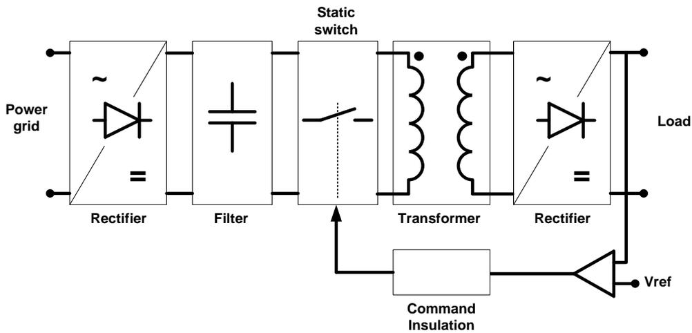
Fig. 1.3 - A switching mode power supply connected to power grid [Ferrieux\_book]
