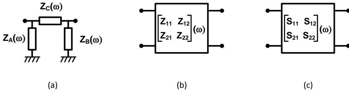
Fig. 2.14 - Frequency dependant two-port models of the inductor
