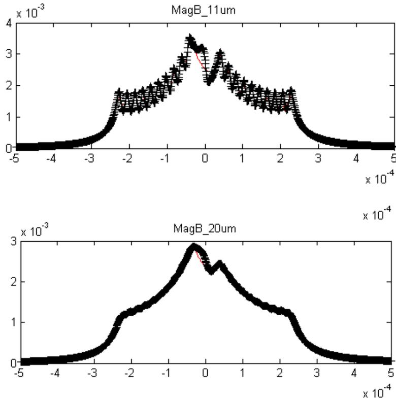
**Fig. 5.11 – Magnetic field created by a square coil along a horizontal axis at 11 and 20  $\mu\text{m}$  from the center computed both with analytical model (*black crosses curve*) and FEA method (*red curve*)**
