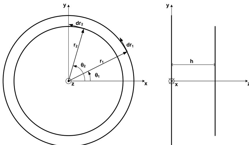
Fig. 3.9 - Two circular wires inductively coupled
