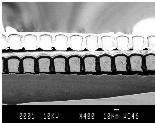
Fig. 4.6 – Cross section view of a two level inductor prototype
