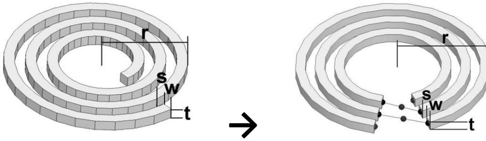
**Fig. 3.1 - Concentric rings approximation of a spiral**
