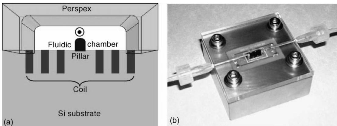
**Fig. 5.3 - A bead trapping microfluidics device realized by the Institute of Microelectronics, the Institute of Bioengineering and Nanotechnology and Nanyang Technological University of Singapore. (a) Schematic drawing of the device with the fluidic chamber capping the coil connection block and (b) final fluidic block with chip inserted in it.**
