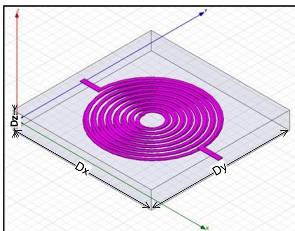
Fig. 3.18 - The inevitable "air box" for FEM simulations
