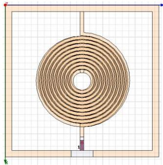
Fig. 3.21 – Top view of the inductor prototype.
