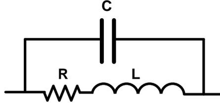
Fig. 2.3 – Lumped elements model of an air inductor
