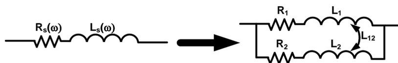
Fig. 2.7 - A way of representing skin and proximity effects with non frequency dependant lumped elements
