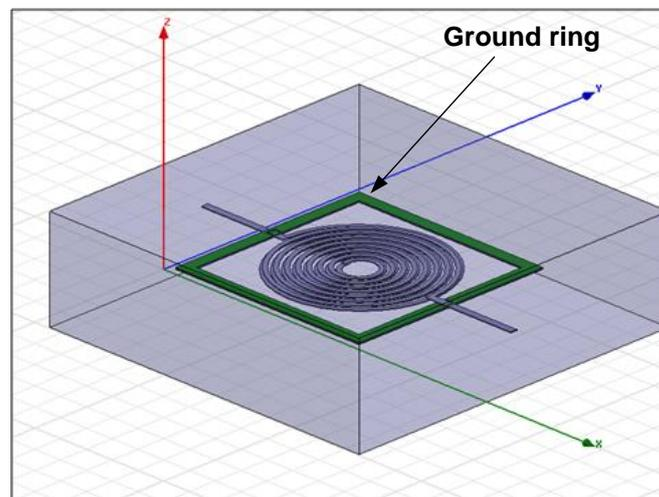
Fig. 3.20 - Simulated inductor with ground ring.
