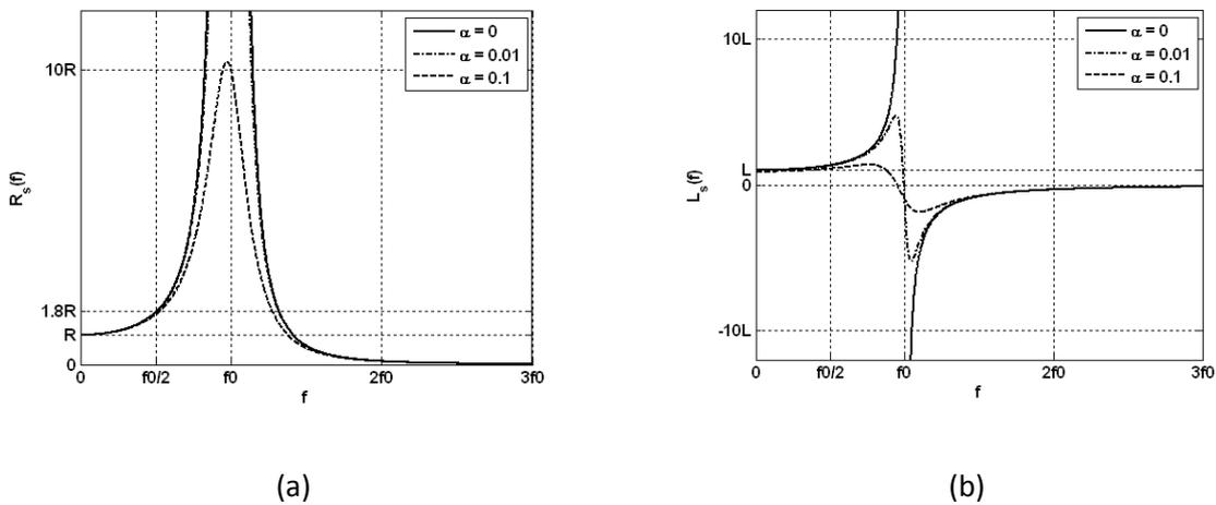
Fig. 2.4 - Normalized representation of real inductor equivalent resistance and inductance versus frequency
