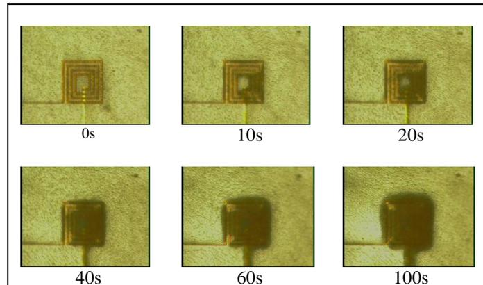
Fig. 5.12 - Images taken from a movie and showing beads stopped by the coil under an intensité  $I = 50 \text{ mA}$
