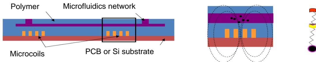
Fig. 5.5 - Microfluidic application of spiral inductor actuator
