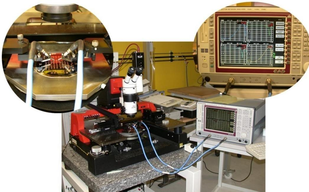
Fig. 4.15 - Vector network analyzer experimental bench
