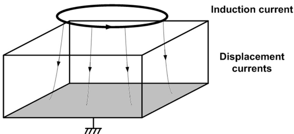
Fig. 2.12 - Displacement currents in the substrate
