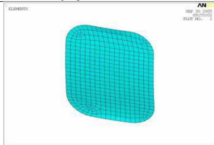
Figure 6 : The shell model of the gap and flush.
