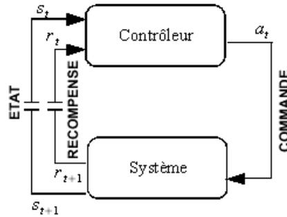
FIGURE 2.1 – Boucle sensori-motrice
