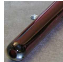
Fig. 2. (b) chalcogenide tube formed by rotational casting
