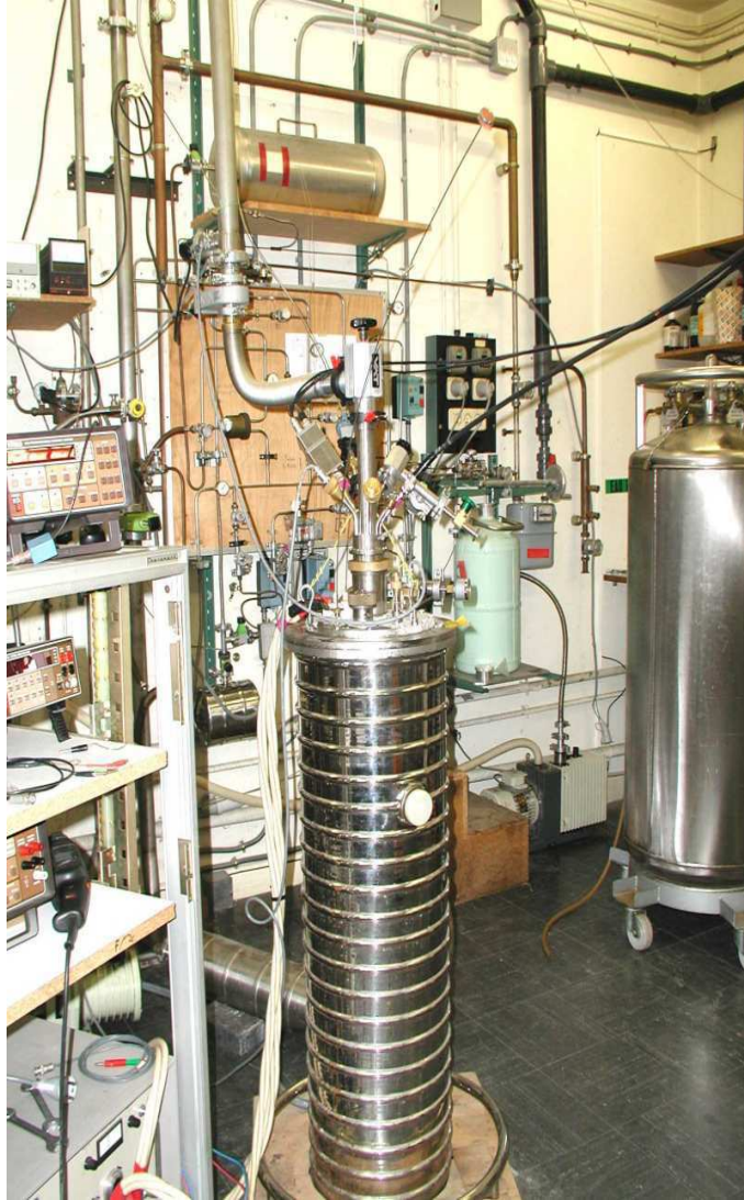
Figure 4.7: Photo of the 35 mK dilution refrigerator.
