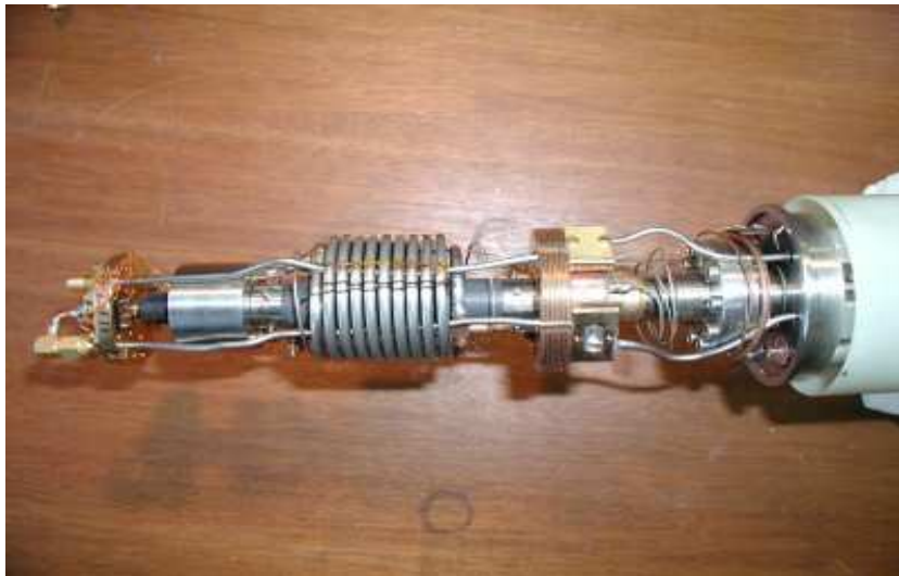
Figure 4.6: The top of the dilution refrigerator probe.
