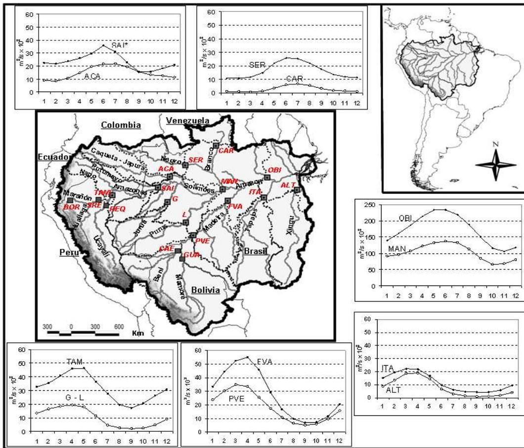
FIGURE 2.1 – Localization of the main sub-basins and hydrological stations of the Amazon Basin. The 1974-2004 mean monthly discharge ( $\text{m}^3/\text{s} \times 10^3$ ) is presented for each sub-basin. G–L data is the sum of Gavião and Labrea stations data. Altamira and Itaituba sub-basins, on the Xingu and Tapajós Rivers respectively, are not part of the Amazon basin in Óbidos. The X axis is from 1 for January to 12 for December. Andean mountainous regions are shaded.
