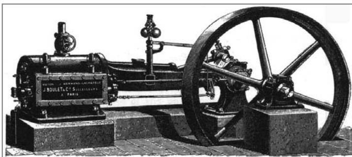
Figure 5 : MACHINE DE TYPE HORIZONTAL [BORGNIIS 1821]
