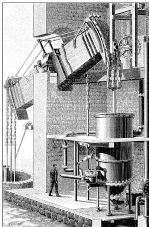
Figure 2 : GRAVURE D'UNE MACHINE DE NEWCOMEN UTILISEE POUR LE POMPAGE DE L'EAU EN 1745 [TISSANDIER 1896]
