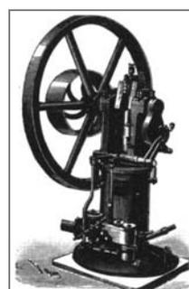
Figure 6 : MACHINE A VAPEUR DE TYPE VERTICAL [BORGNIIS 1821]
