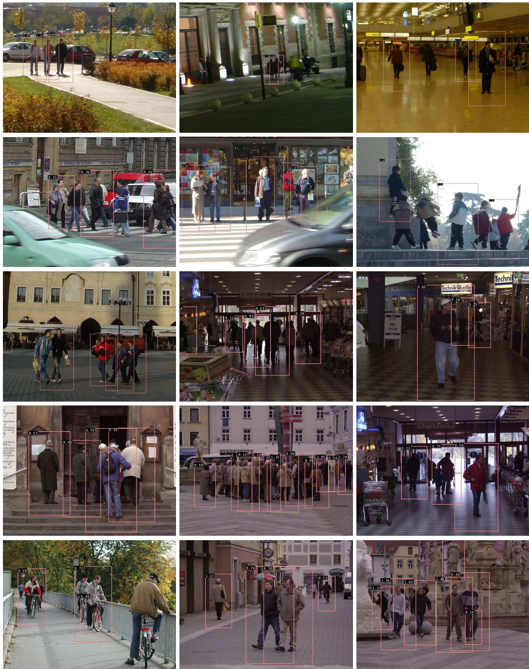
Fig. 5.6. Some examples of detections on test images for the final person detector. The detector is able to detect people in crowds in varied articulated poses with different clothing, background clutter and illumination. Some images also show missed detections and/or false positives. The threshold used to display the detections in this figure corresponded to a recall rate of 0.7 at a precision of 0.75.
