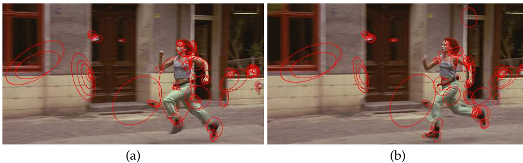
Fig. C.1. Inconsistent behaviour of key point detectors on humans. (a) Detected key points by the Harris-Laplace detector [Mikolajczyk and Schmid 2004] for one frame of a video sequence. (b) Detected key points for the next frame of the sequence. Note that although the detector fires reliably for the same points in the background, it fails to perform consistently on the similar locations for the person.
