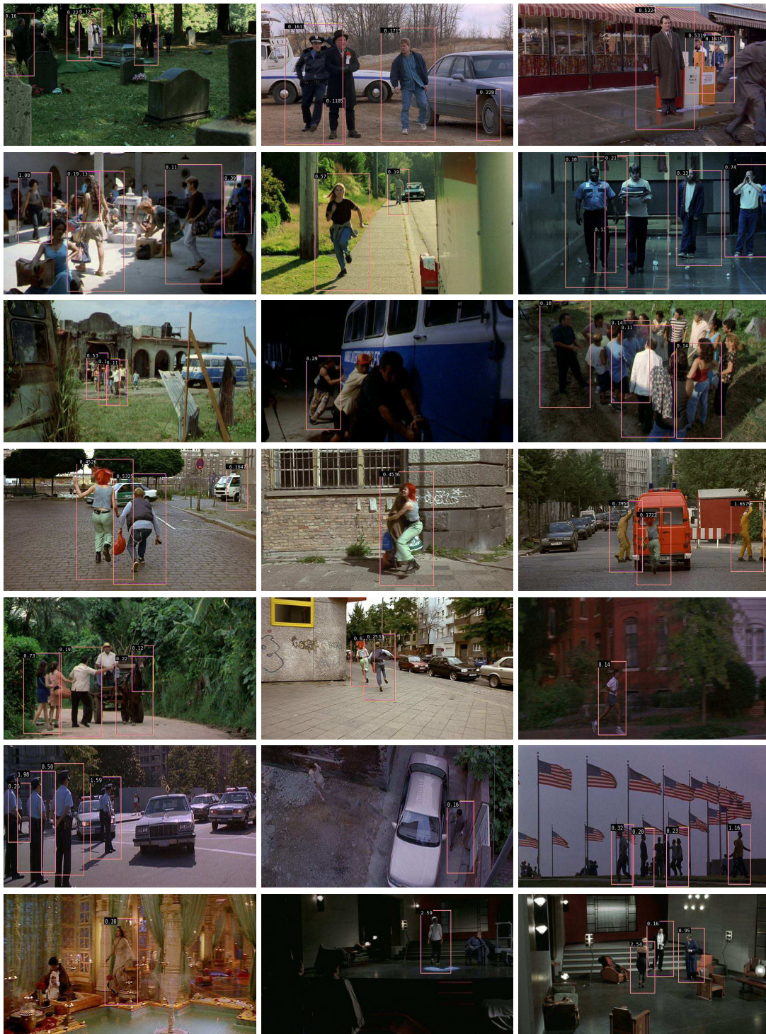
Fig. 6.8. Sample detections on Motion Test Set 2 from the combined R-HOG + IMHmd detector trained on Set 1 + Static. Note the variations in pose, appearance, background and lightning. Certain poses, such as people pushing the bus (3 th row, 2 nd column), fish eye lens views (3 th row, 3 th column), and views of people from the top (6 th row, 2 nd column) were not seen in the training set. The detector sometimes has false positives on legs (1 st row, 2 nd column) and on tyres with relatively oblique views.
