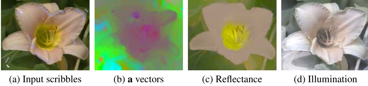
Figure 7.5: (a) The user can specify pixels sharing a constant reflectance (blue), a constant illumination (red), or a fixed illumination (white). Each type of scribble is represented with a single color for illustration purpose, while in our implementation strokes of similar color share the same constraint. (b) Visualization of the \mathbf{a} vectors that vary across the image to fit the user constraints. (c,d) Resulting reflectance and illumination.
