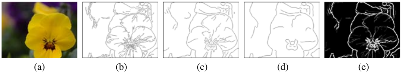
Figure 2.5: Edge importance. (a) The input image. (b-d) Canny edges at increasing scales. (e) The lifetime measure reflects the importance of edges: “older” edges correspond to more stable and important structures.
