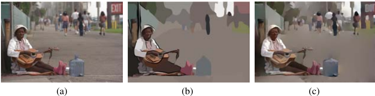
Figure 2.14: Comparison with the DeCarlo et al. [DS02]. (a) Original picture. (b) DeCarlo et al. results exhibit flat color regions. (c) Our result simplifies the image while keeping smooth color variations.
