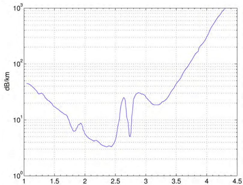
Figure 3.17 - Transmission of the L-band single-mode fibre (in dB/km) vs. wavelength (in \mu\text{m} ; courtesy VerreFluoré).
