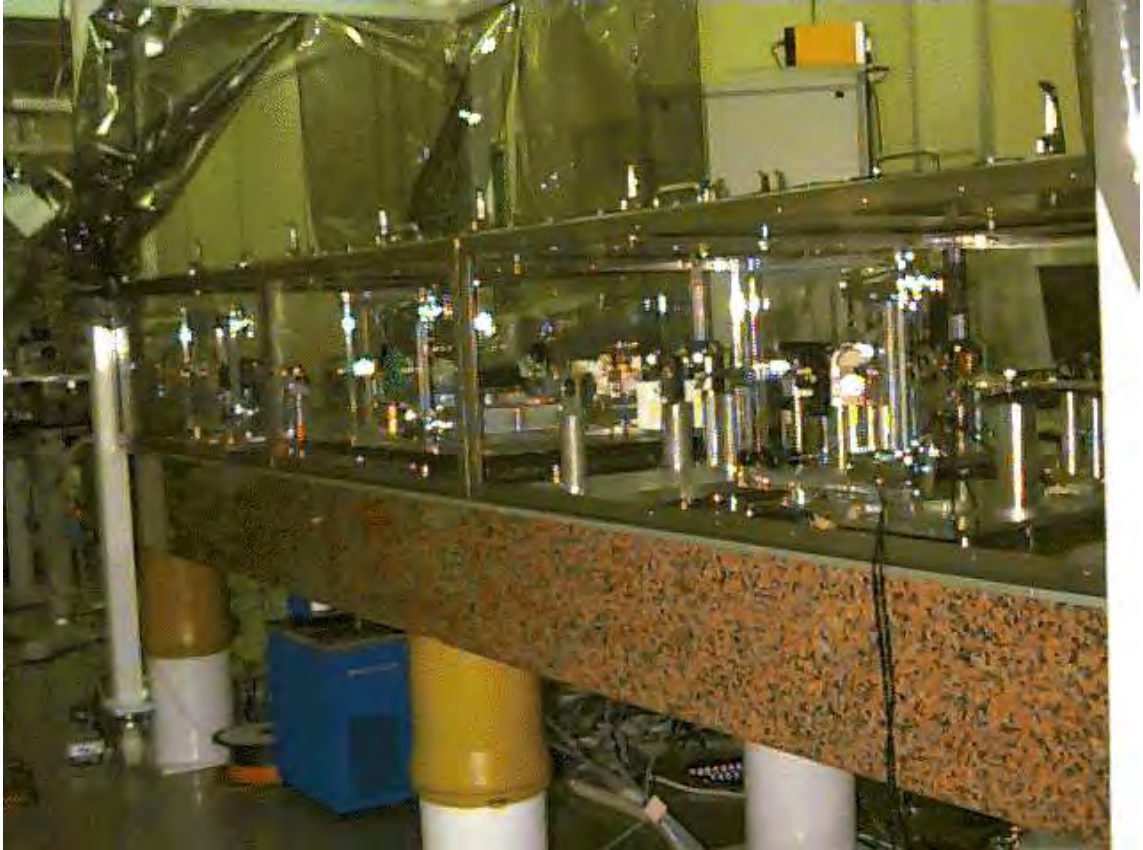
Figure 3.1 - A global view of the first nulling testbed at the Institut d'Astrophysique Spatiale (Ollivier 1999). It operated at ambient temperature in monochromatic polarised light at 10.6 \mu\text{m} and achieved nl = 7 \times 10^{-4} .
