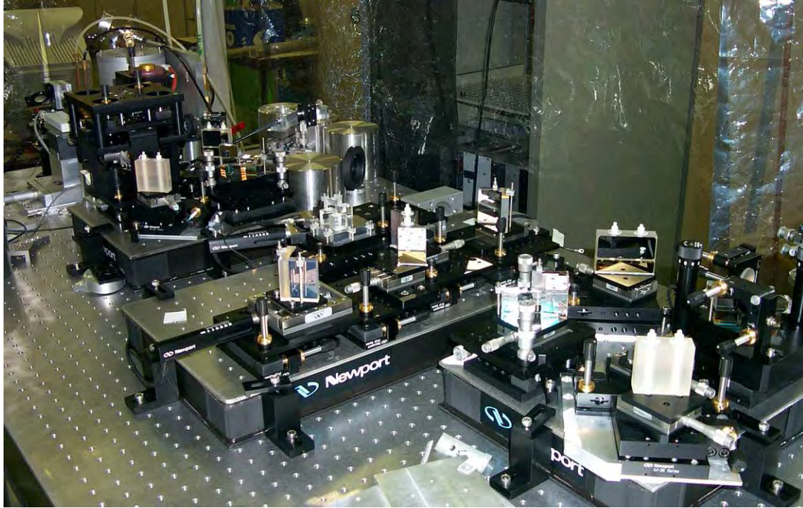
Figure 3.2 - A view of the SYNAPSE nulling testbed's interferometric setup (Brachet 2005, photograph taken in Sept. 2003).
