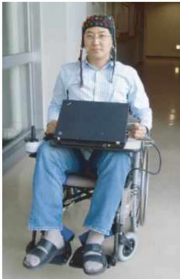
Figure 2.10: With the Toyota/Riken's brain controlled wheelchair, the user continuously controls the velocity of the wheelchair by imagining left hand, right hand or both feet movements (from [59]).
