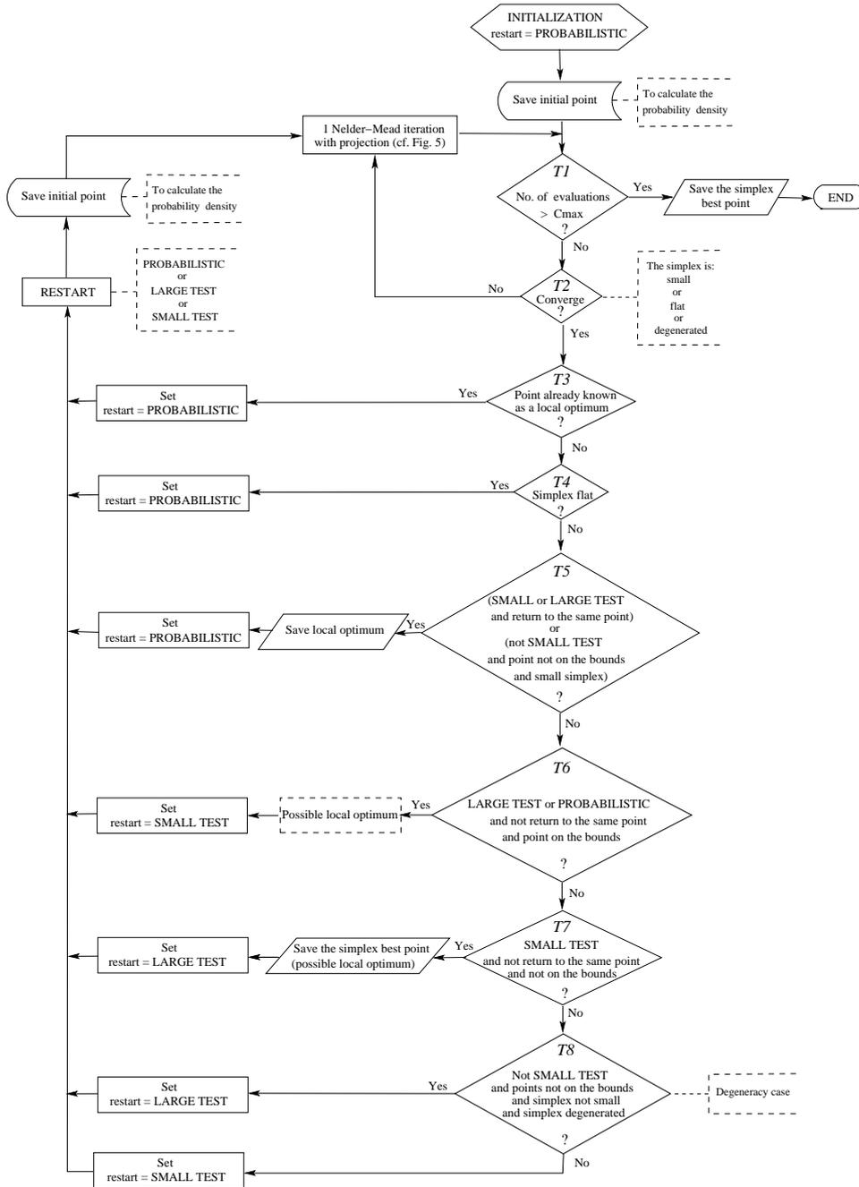
Figure 1.15: Restarts and convergence tests linking in GBNM
