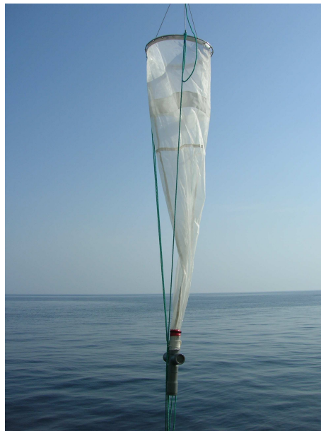
Figure 2.3: A picture of the zooplankton WPII net used onboard MOUTON 2007 survey.
