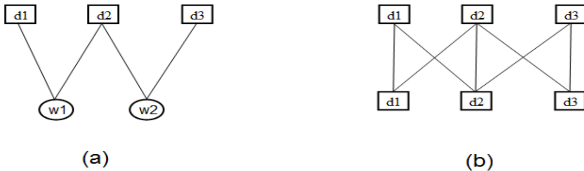
Figure 3.9 A sample graph corresponding to (a) the adjacency matrix \mathbf{A} , and (b) the adjacency matrix \mathbf{L}
