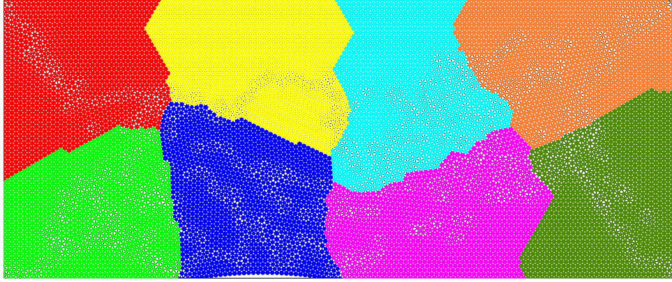
Figure 2.8: Partition of graph BUMP into 8 parts with SCOTCH 4.0, using the multilevel framework with a Fiduccia-Mattheyses refinement algorithm. The cut is equal to 714 edges. Segmented frontiers are clearly evidenced, compared to Figure 4.12, page 50.
