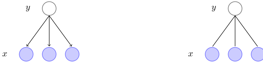
Figure 2.1: Graphical representations of the generative model naive Bayes (left) and discriminative model logistic regression (right).
