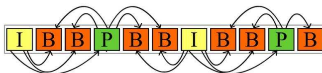
Figure 5.1: Video compression: each P frame is produced from I frame, each B frame is produced from I and P frames.
