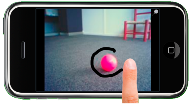
Fig. 4. Encircling an object allows the user to notify the robot that he wants to teach a name for this object. But it also provides an useful rough object segmentation.
