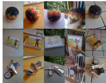
Fig. 10. Several examples of a specially constructed objects database corresponding to the kind of objects we think an human would like to teach to its robot (everyday object, small and carryable). The images were taken with different backgrounds in order to be able to recognize objects in spite of their location.
