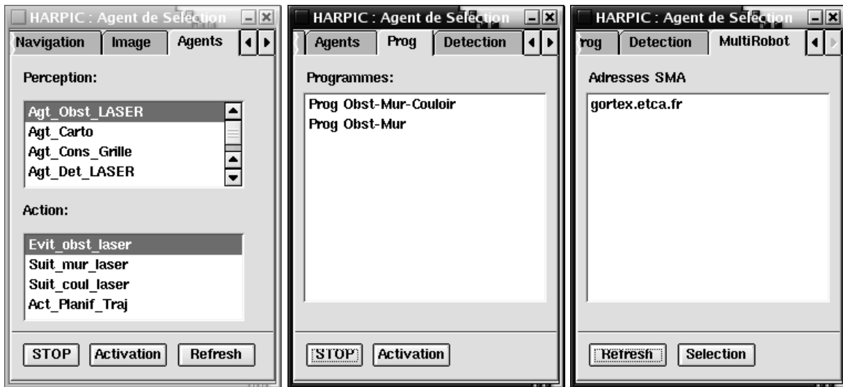
Figure 4. Interface for agent (left), program (center) and robot (right) selection.
