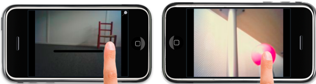
Fig. 3. Drawing attention towards an object: the user first sketches directions to position the robot such that the object is in its field of view (left), and if he wants to center the robot's sight on a specific spot just tap on it (right).
