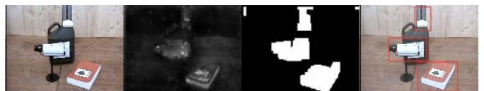
Figure 4. Steps of image segmentation : the first image is the original image taken by the robot, second is the saliency map computed on the subsampled image, third is the saliency map once thresholded and passed through region growing and fusion algorithm. The last one shows the salient regions drawn on the original image
