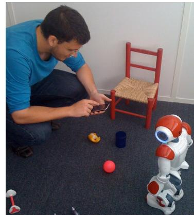
Fig. 1. Using a handheld device as a mediator object to control the movements of a social robot.
