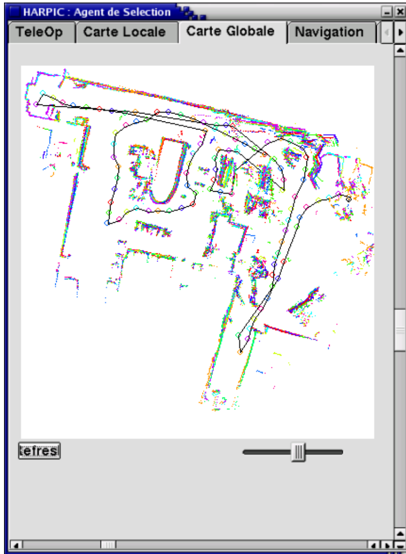
Figure 7. Map and robot trajectory generated during a JNRR'03 demonstration in the IFMA hall. Each circle on the robot trajectory represents the diameter of the robot which is about 50 cm.
