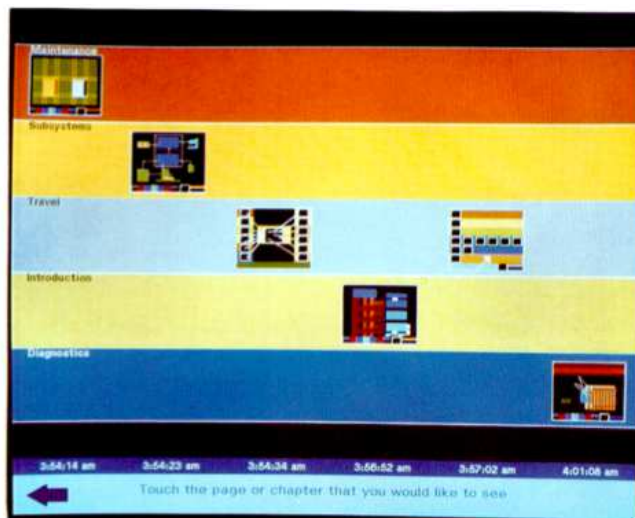
Fig. 7. The timeline page. Miniatures of the most recently viewed pages appear in chronological order. Each is nested in a colored band associated with its parent chapter. Touching a page takes the reader back to that page. The arrow at the bottom scrolls the display so the reader may examine pages that were seen earlier in the session.
