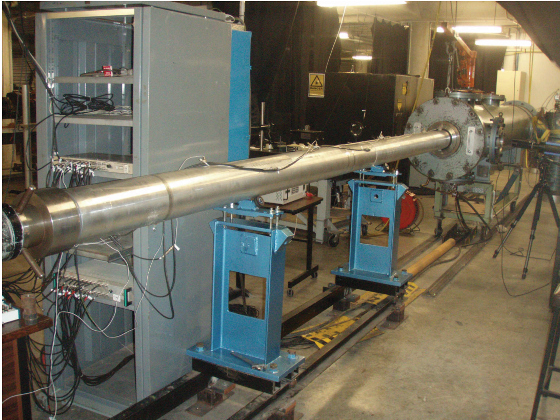
Figure 3.5 : Photograph of the modified X2 facility in NRST-Al mode. Image shows the aluminium shock tube and the dump tank with the optical systems in place.
