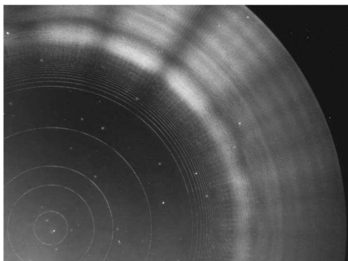
FIG. 6.—Image of the binary mask taken with a microscope. The transmission is about 10% on the edge of the pupil.
