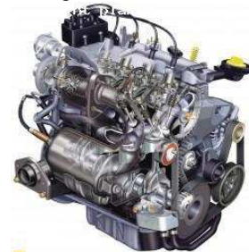
Fig. 1: D4FT: 1.2 liter turbocharged gasoline engine The engine main characteristics are shown in Table 1 and the schematic description of the air path in Fig. 2. Control inputs are throttle’s and waste-gate’s valves. Both control inputs are necessary: in broad strokes, throttle’s valve is used for low pressure references and waste-gate’s valve is needed when the reference pressure is higher than 1 Bar.
