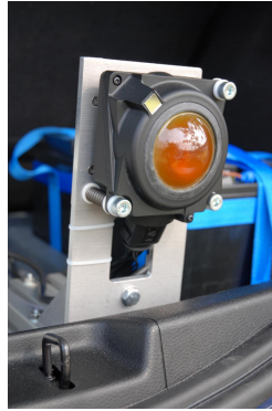
Figure 4: Radar Autocruise ACC.
