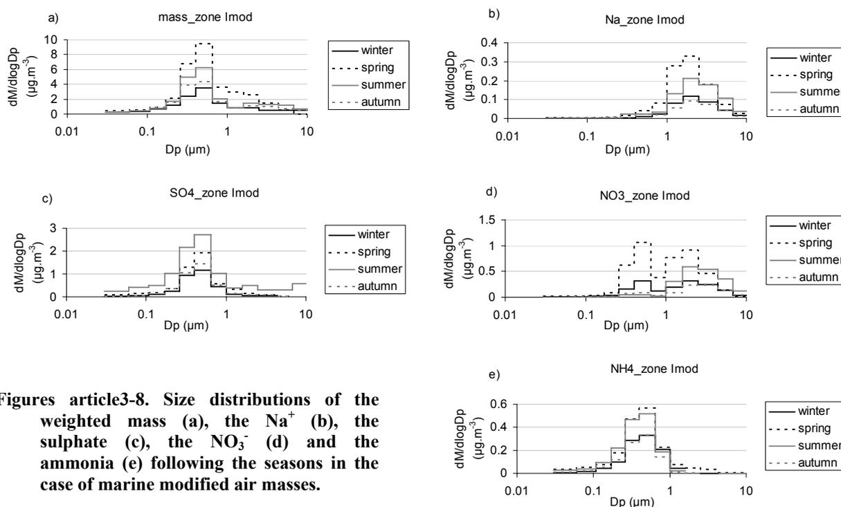
**Figures article3-8. Size distributions of the weighted mass (a), the  $\text{Na}^+$  (b), the sulphate (c), the  $\text{NO}_3^-$  (d) and the ammonia (e) following the seasons in the case of marine modified air masses.**
