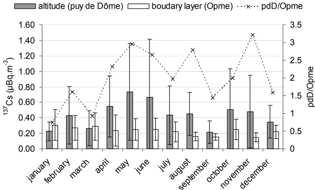
Figure article1-4. Monthly mean of the 3-years period  $^{137}\text{Cs}$  activity levels at Opme and the puy de Dôme on the left axis and the ratio pdD/Opme on the right axis. The y-errors bar is the standard deviation.
