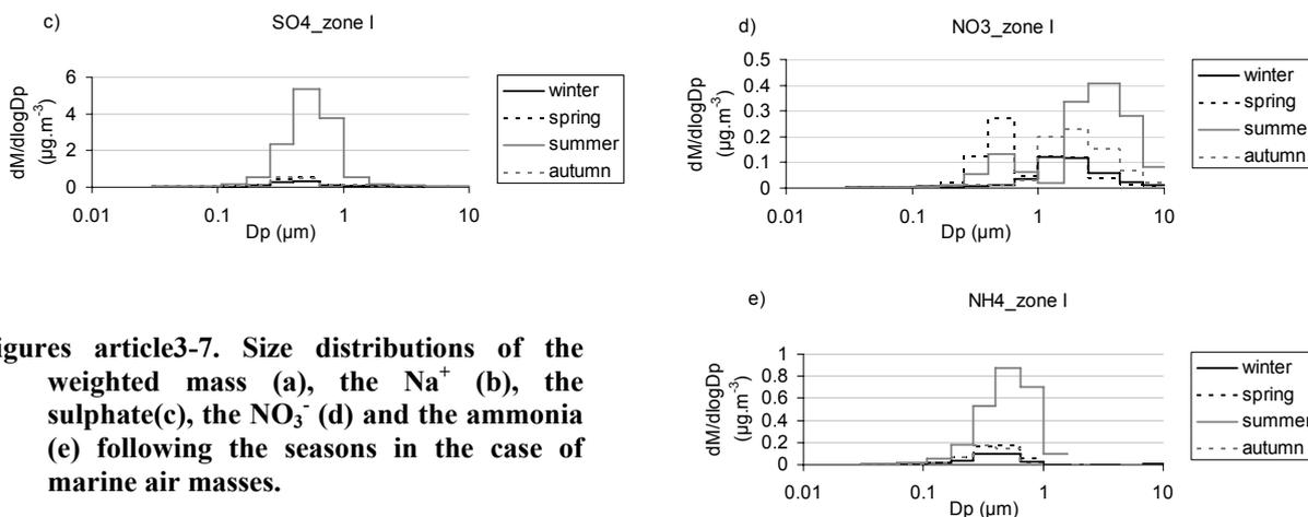
**Figures article3-7. Size distributions of the weighted mass (a), the Na<sup>+</sup> (b), the sulphate(c), the NO<sub>3</sub><sup>-</sup> (d) and the ammonia (e) following the seasons in the case of marine air masses.**
