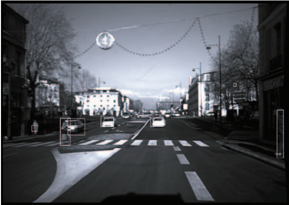
Fig. 14. This scene is more complex than the previous ones, as there are many targets, moving in different directions. However, our method extract them all. The vehicles in the background aren't detected because a minimum disparity under which data is not processed is set. This was done in this sequence only, because of the many moving vehicles in the background.
