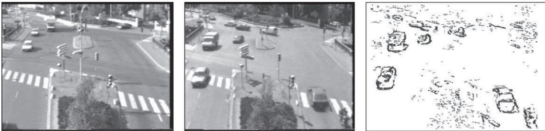
Fig. 6. (top left) Sequence of images used to build the references; (top middle) sequence of images used to test the detection (shot 6 months before the top left sequence) and (top right) detection obtained using our method.
