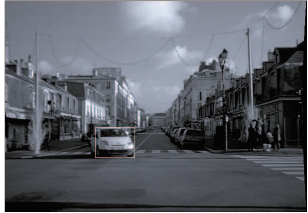
Fig. 12. This image is extracted from a different sequence, the stereo sensor is moving forward and turning to the left. The white car is well defined and detected. On the other hand the pedestrians on the right are standing still. A stereo-only detection algorithm would have detected them as potential obstacles in spite of they are on the sidewalk.
