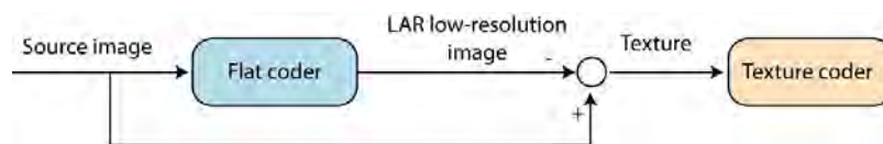
Figure 2.1: General scheme of two-layer LAR coder
