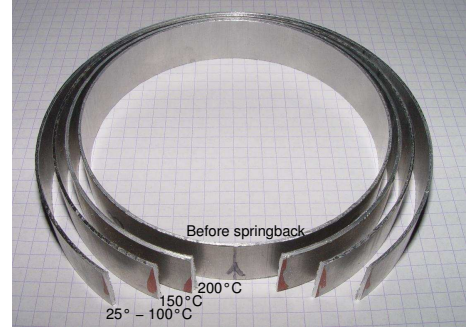
FIGURE 4.4 – Opening of the rings for several temperatures in the range 25 - 200^\circ\text{C} .
