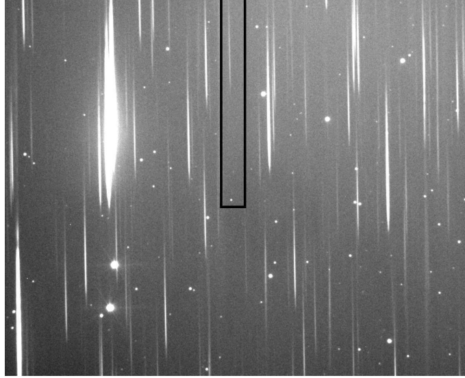
Figure 2.3: The field of quasar PG1634+706 (north is at bottom of the figure). The object and its spectrum are surrounded by a rectangle. In this image it can be distinguish the zero order (objects are dots) and the first order (light is dispersed) - Popescu et al. [2012a].
