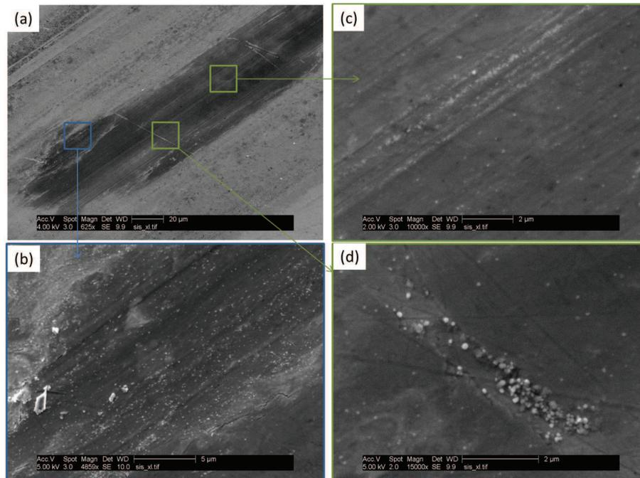
FIGURE 3.31 – SEM micrographs at different magnifications of the centre of the wear track. The observed tribofilm is formed through boundary friction of a PAO6+1%  $IF - WS_2$  in a steel/steel contact.
