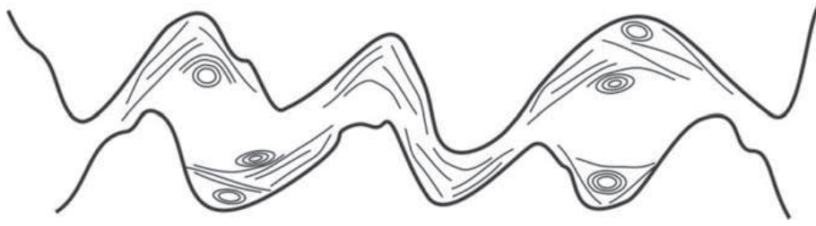
FIGURE 1.8 – Schematic presentation of nanoparticle deposition in the valleys of the surfaces which increases the real contact area. Micro-grooves (roughness valleys) act as reservoirs and help to preserve the nanoparticles within the contact [46]
